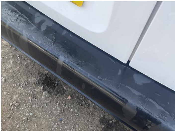
1: Bumper Rear Moulding Scuffed (Unpainted) UpTo 100mm
