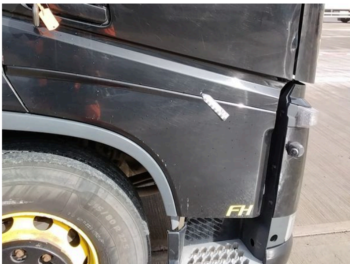
14: Door osf Chipped Over 5mm
