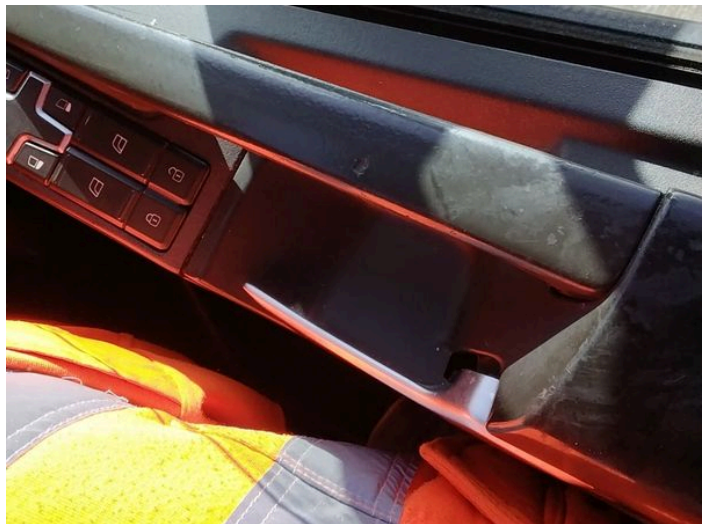
20: Handle Inner osf Damaged Replace
