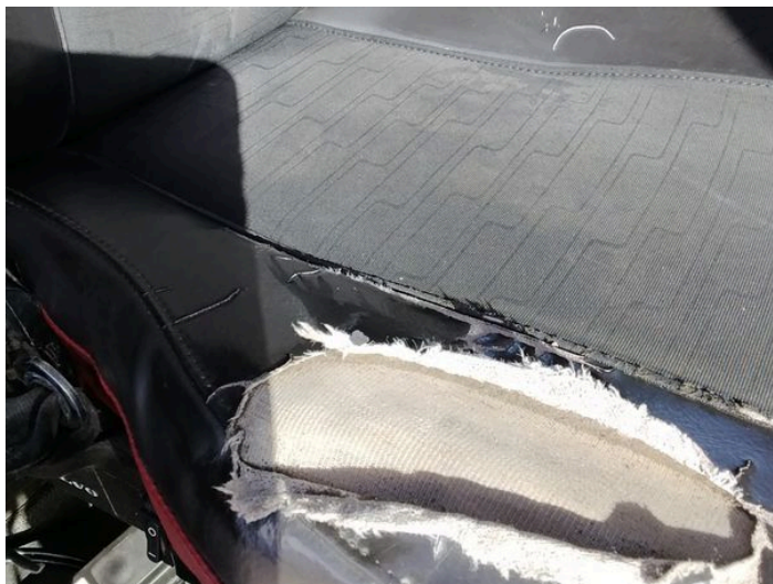
21: Seat Base Cover osf Torn Over 3mm
