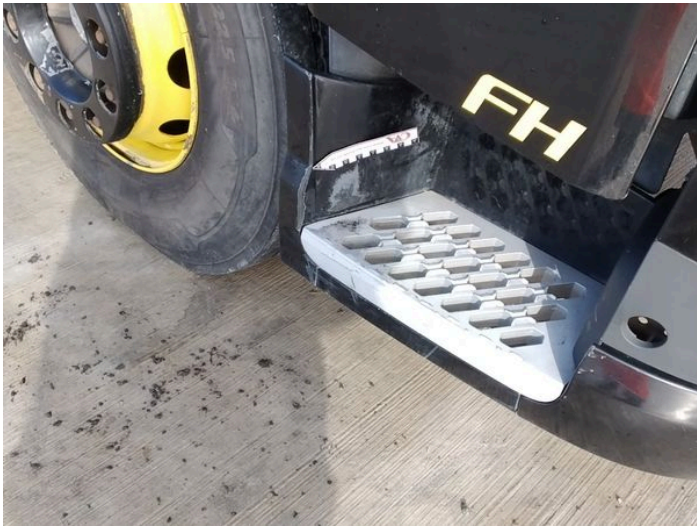
17: Wing Front Arch Extension os Scratched (Painted) Over 25mm Thru Paint
