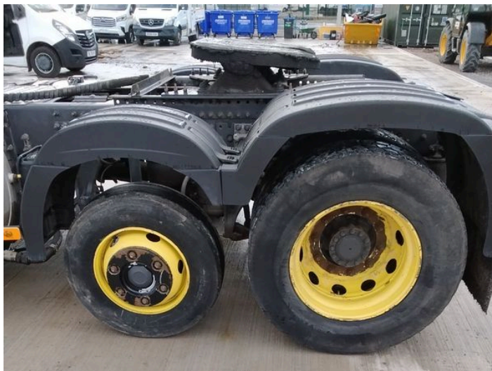
9: Wheel nsr Corroded Light
