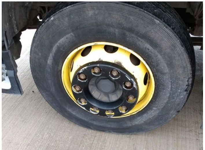
8: Wheel nsf Corroded Light
