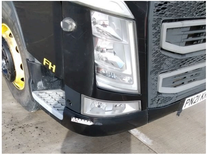
18: Bumper Front Scratched Over 100mm Thru Paint
