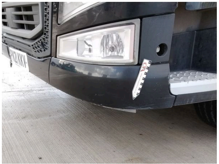
4: Bumper Front Scratched Over 100mm Thru Paint
