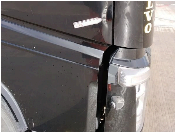
15: Door osf Dented Over 30mm
