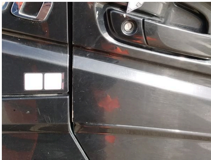
22: Handle Outer osf Scratched (Painted) Over 25mm Thru Paint
