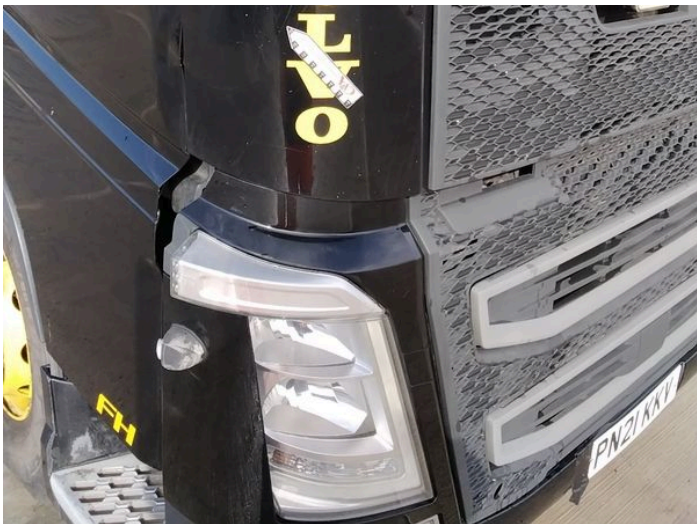
19: Panel Front Chipped Over 5mm
