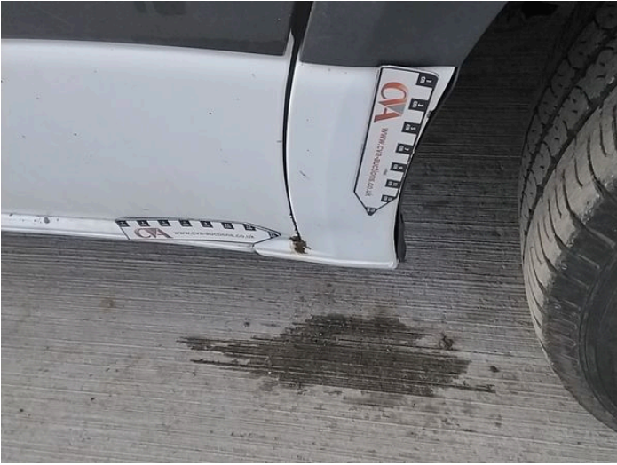
14: Wing osf Dented Over 30mm
