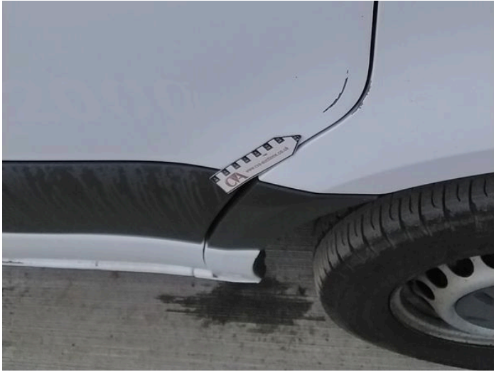
13: Door osf Dented With Paint Damage
