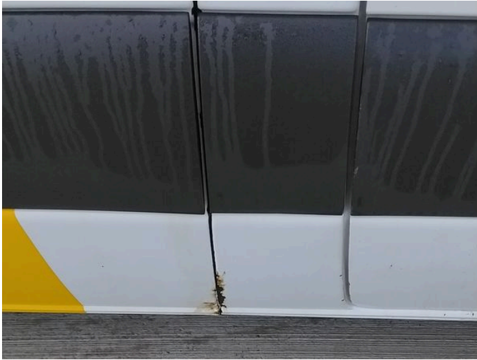
11: B Post os Rusted Over 5mm
