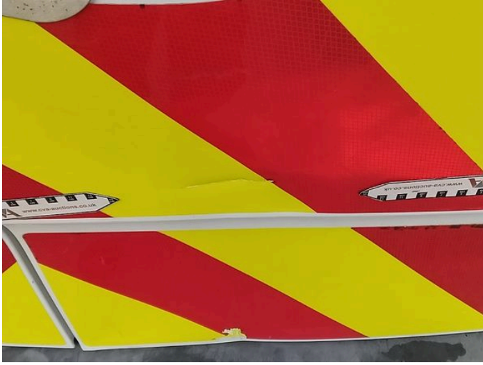
7: Door osr Dented With Paint Damage
