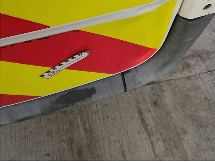
8: Door osr Dented Over 30mm
