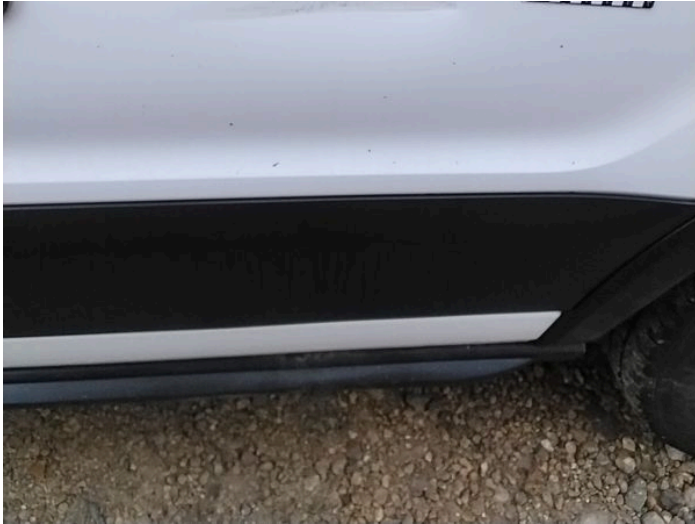
1: Door osf Dented With Paint Damage
