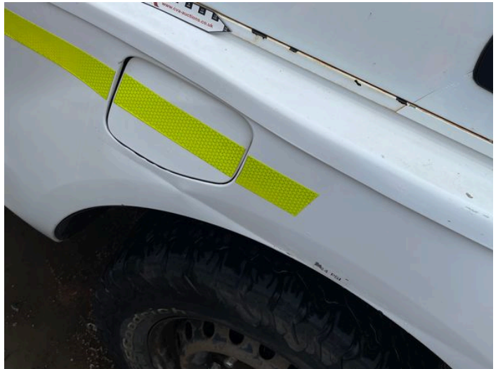
12: Qtr Panel nsr Rusted Over 5mm
