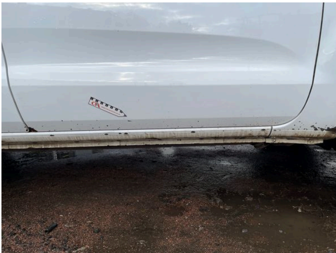
7: Sill os Rusted Over 5mm
