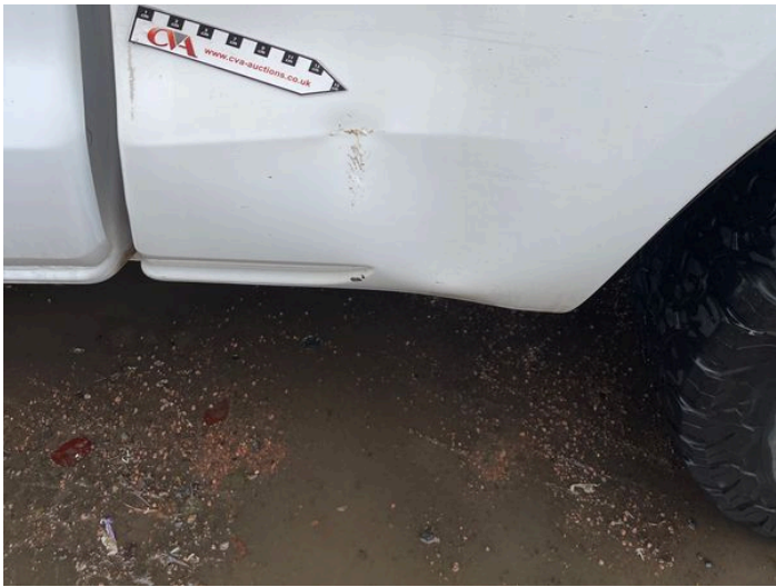
15: Qtr Panel nsr Dented With Paint Damage
