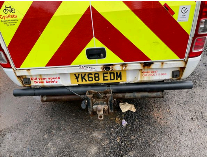
11: Tailgate Rusted Over 5mm
