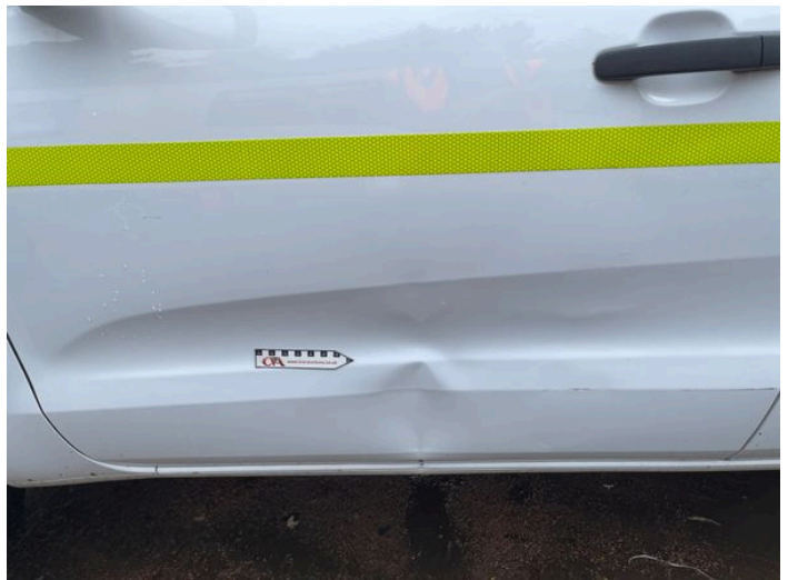
14: Door nsf Dented Over 30% Of Panel
