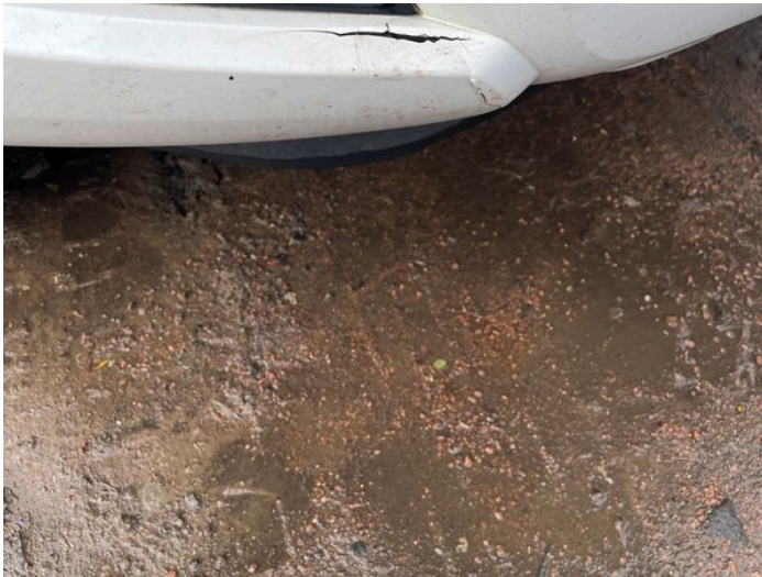
5: Bumper Front Cracked Over 25mm
