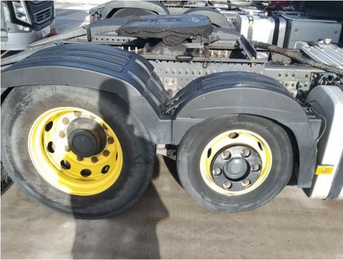
11: Wheel osr Corroded Light
