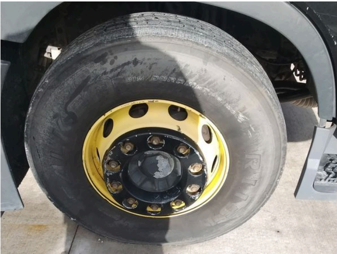
14: Wheel osf Corroded Light
