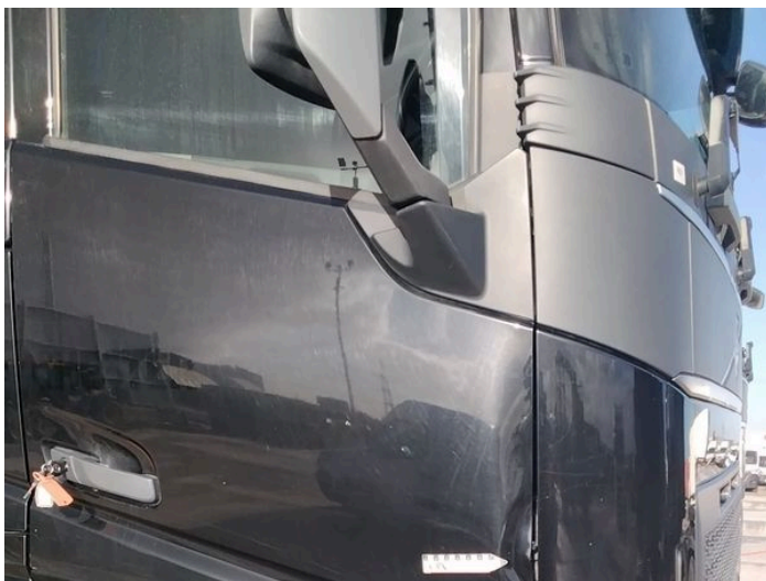
18: Door osf Dented Over 30mm
