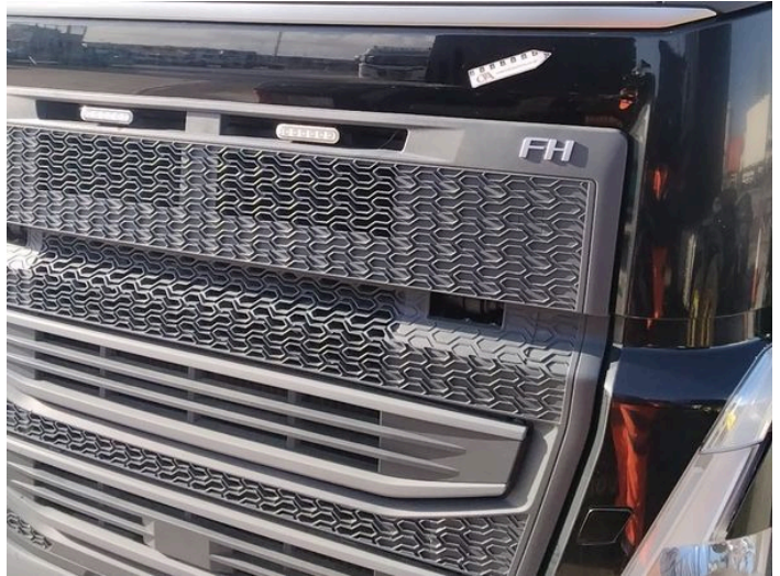
2: Panel Front Chipped Over 5mm
