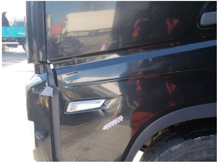
6: Door nsf Scratched Over 25mm Thru Paint
