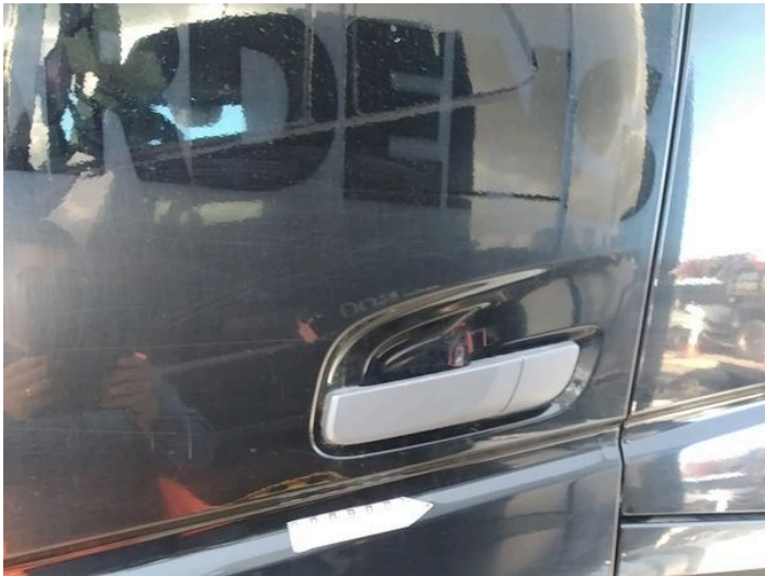
23: Door nsf Dented Over 30mm
