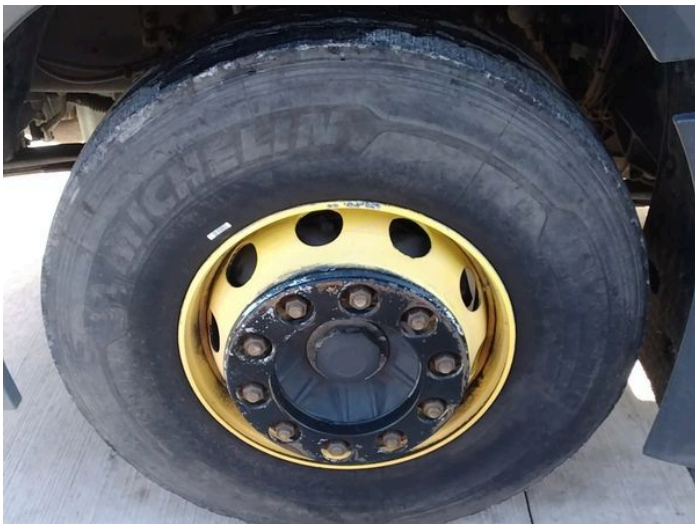
7: Wheel nsf Corroded Light
