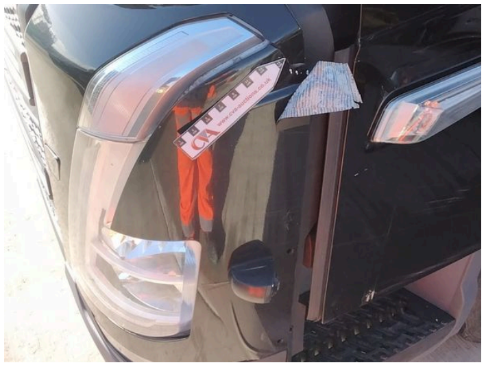
4: Wing nsf Cracked Replace
