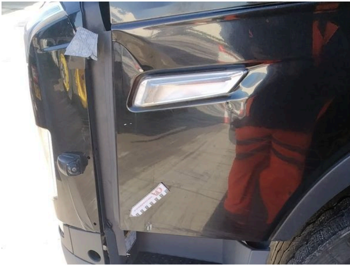
5: Door nsf Dented Over 30mm
