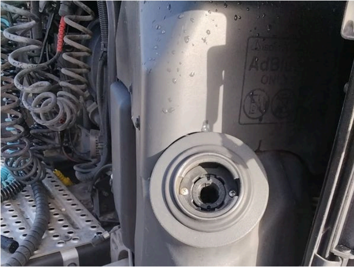
12: Fuel Flap Missing Replace
