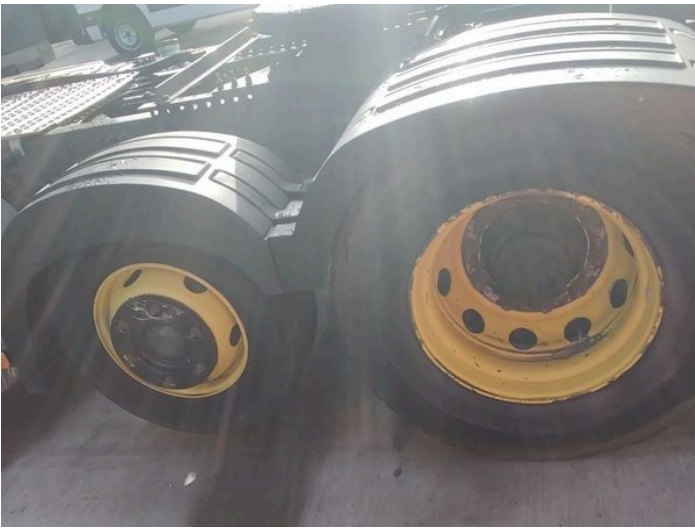
10: Wheel nsr Corroded Light
