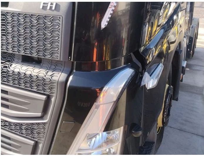
3: Wing nsf Chipped Over 5mm
