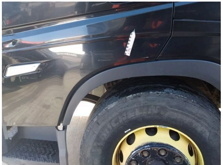
8: Door nsf Chipped Over 5mm
