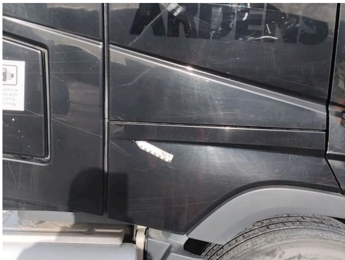
15: Qtr Panel osf Chipped Over 5mm
