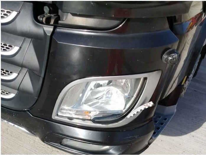
5: Fog Lamp Surround ns Scratched (Painted) Over 25mm Thru Paint
