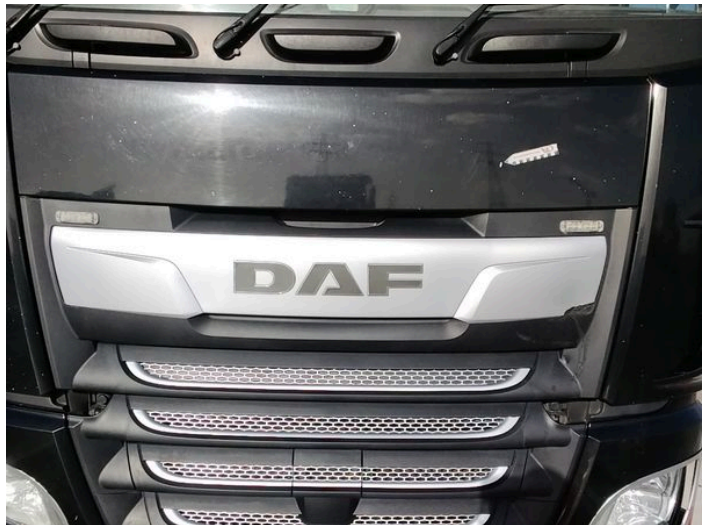
2: Panel Front Chipped Over 5mm
