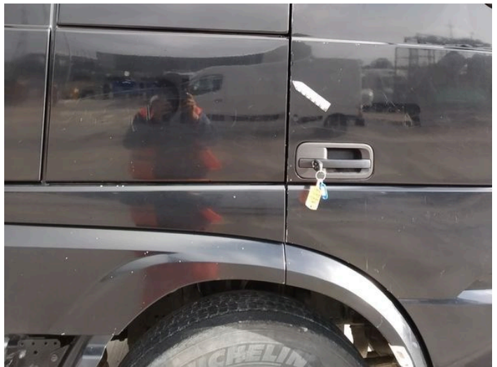
20: Door osf Chipped Edge Chip
