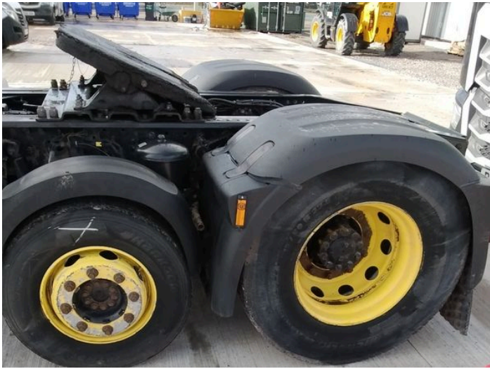
13: Wheel nsr Corroded Light
