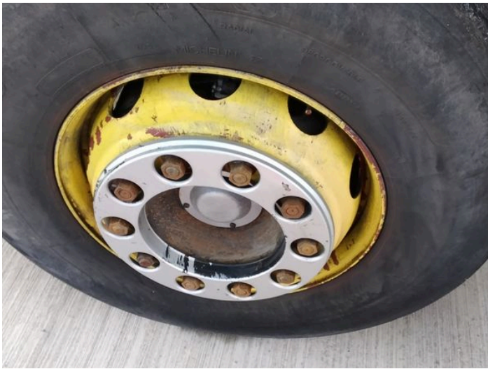
10: Wheel nsf Corroded Light
