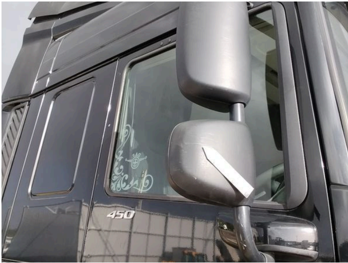
23: Door Mirror Assy osf Scuffed (Unpainted) Over 100mm
