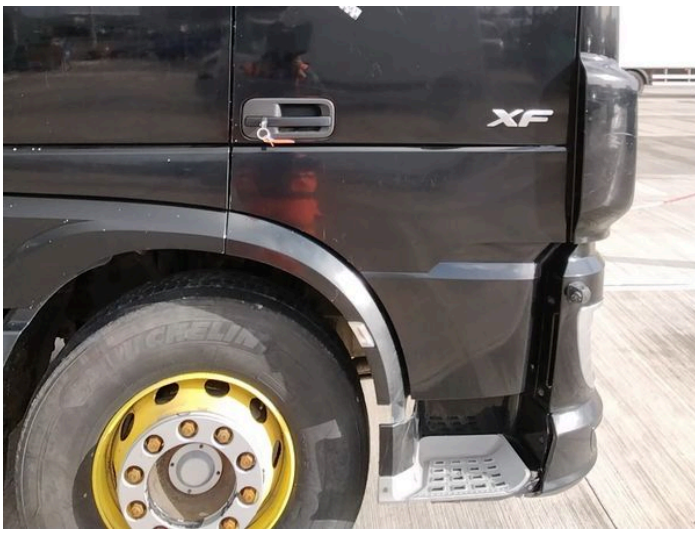
21: Door osf Chipped Over 5mm
