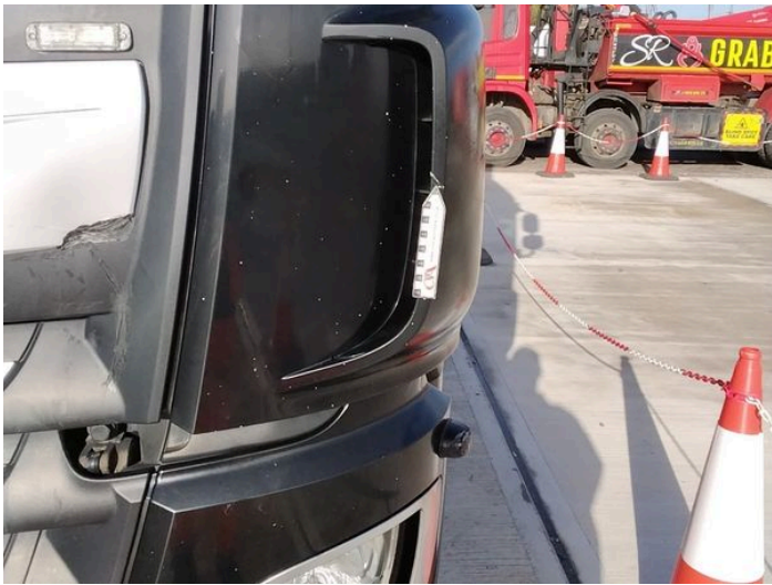
3: Wing nsf Cracked Replace
