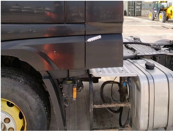
12: Qtr Panel nsr Chipped Over 5mm
