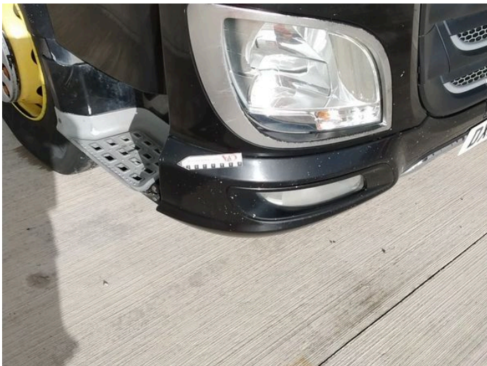
25: Bumper Front Chipped Over 5mm
