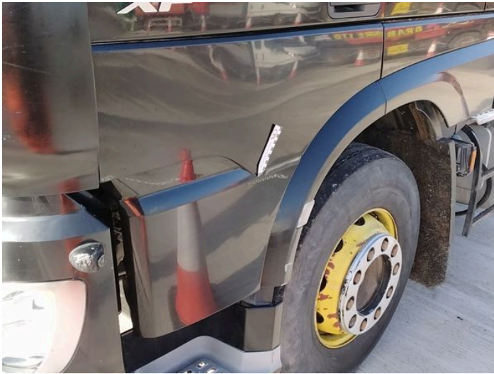
6: Door nsf Scratched Over 25mm Thru Paint
