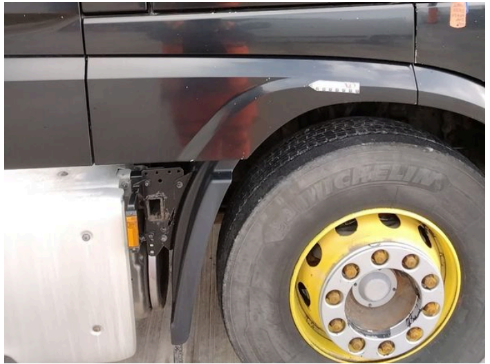
18: Wing Front Arch Extension os Scratched (Painted) Over 25mm Thru Paint
