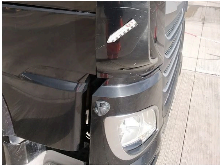
24: Wing osf Cracked Replace
