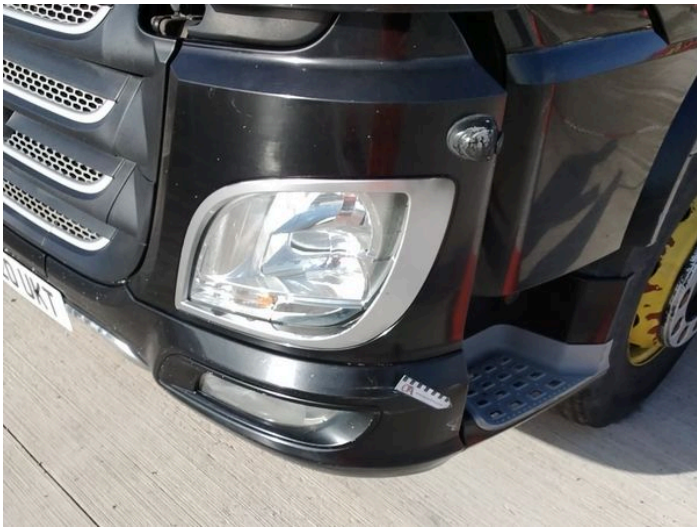
4: Bumper Front Scratched Over 100mm Thru Paint
