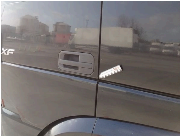
11: Door nsf Chipped Edge Chip
