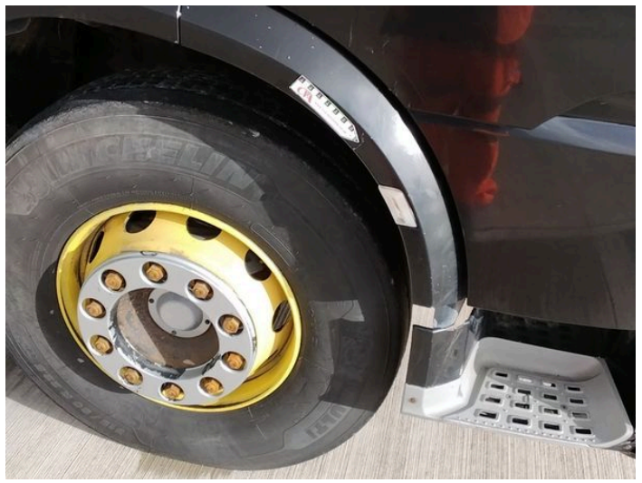
22: Wing Front Arch Extension os Broken Replace
