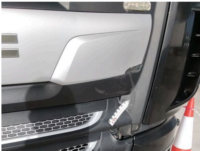
27: Grille Front Broken Replace
