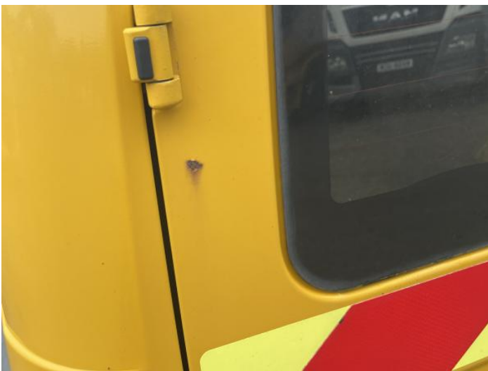
7: Tailgate Rusted Over 5mm
