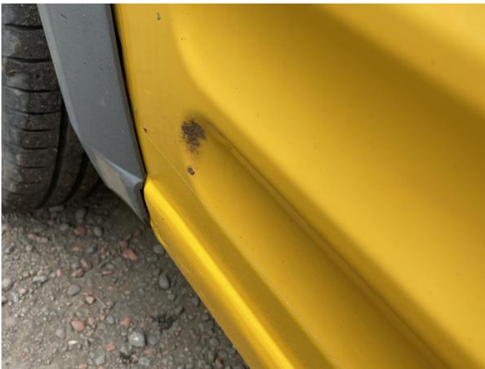
5: Qtr Panel osr Rusted Over 5mm
