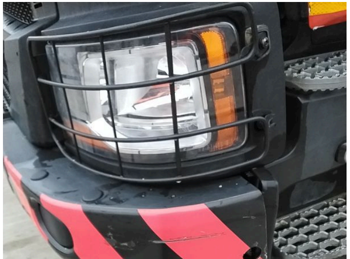
2: Bumper Front Scratched Over 100mm Thru Paint
