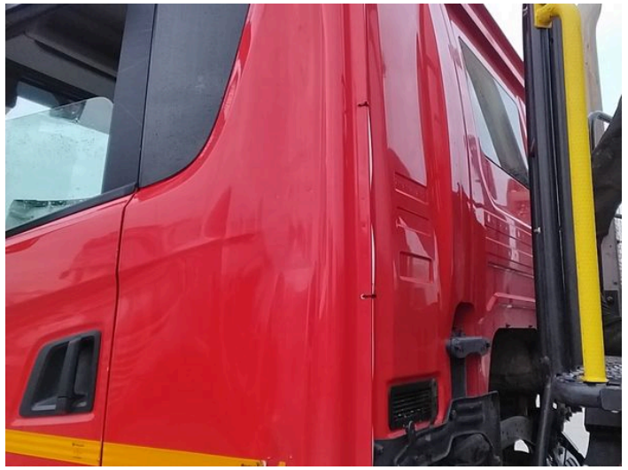
4: B Post ns Dented With Paint Damage
