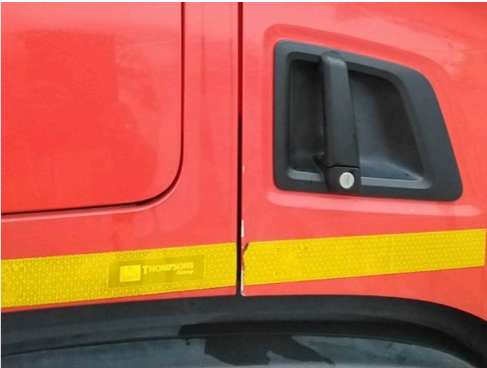
5: Door osf Scratched Over 25mm Thru Paint
