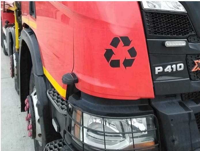
1: Panel Front Dented With Paint Damage
