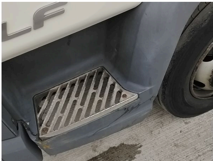
3: Wing nsf Cracked Replace
