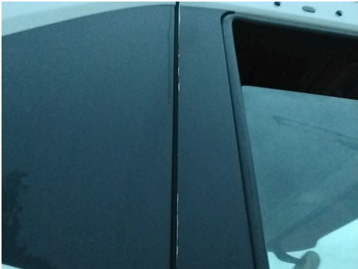
6: Door osf Scratched Over 25mm Thru Paint
