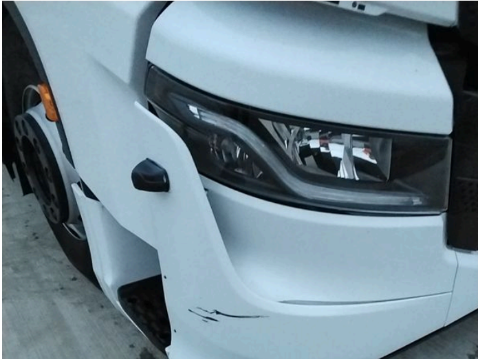
1: Bumper Front Scratched Over 100mm Thru Paint
