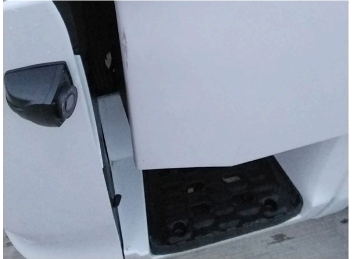
2: Door Moulding nsf Scratched (Painted) Over 25mm Thru Paint
