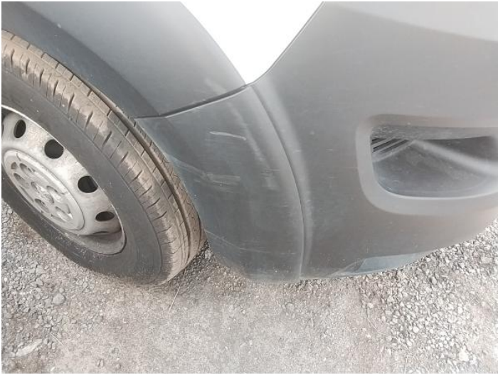
27: Bumper Front Moulding Scuffed (Unpainted) Over 100mm
