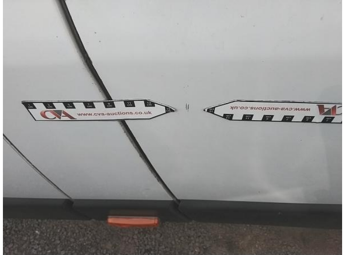
22: Door osf Dented With Paint Damage
