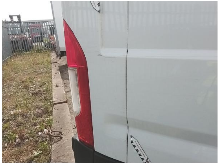
18: C Post os Scratched Over 25mm Thru Paint
