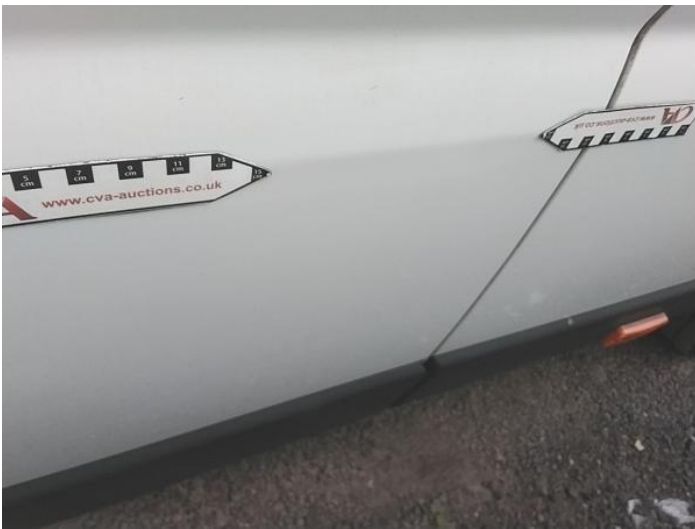
5: Qtr Panel nsr Dented Over 30mm
