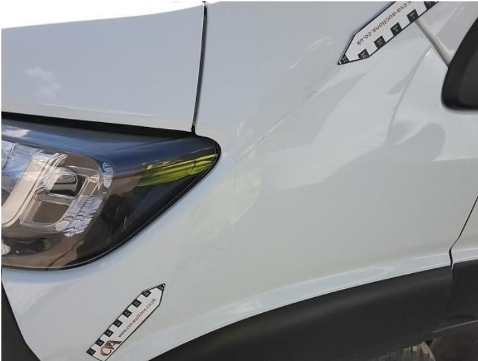
3: Wing nsf Scratched Over 25mm Thru Paint
