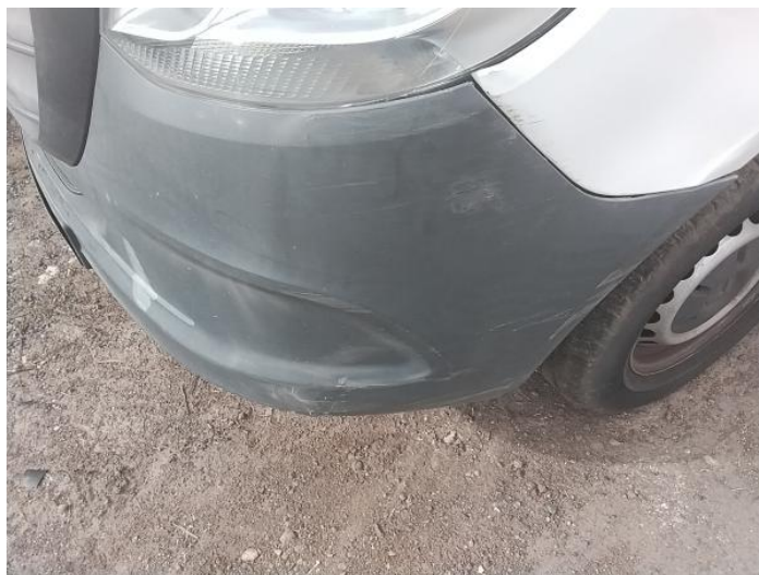
2: Bumper Front Scratched Over 100mm Thru Paint
