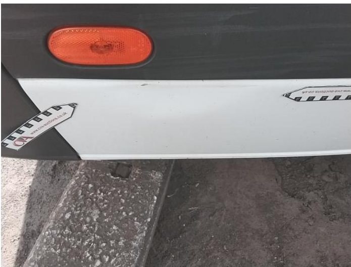
25: Qtr Panel osr Dented With Paint Damage
