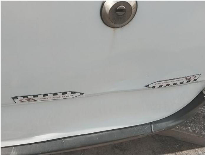
21: Door osr Dented Over 30mm
