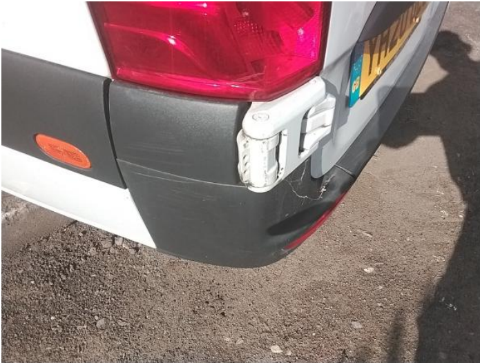
15: Bumper Rear Moulding Scuffed (Unpainted) Over 100mm
