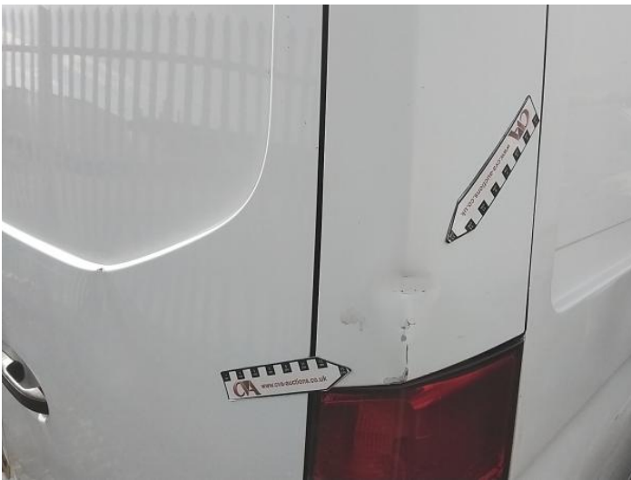
23: C Post ns Dented With Paint Damage
