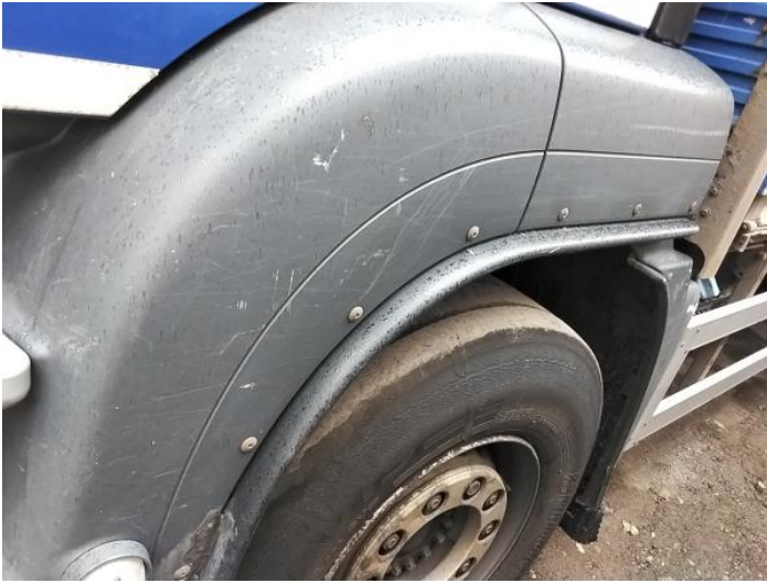
3: Wing nsf Scratched Over 25mm Thru Paint
