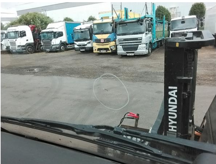
7: Screen Front Chipped Over 10mm
