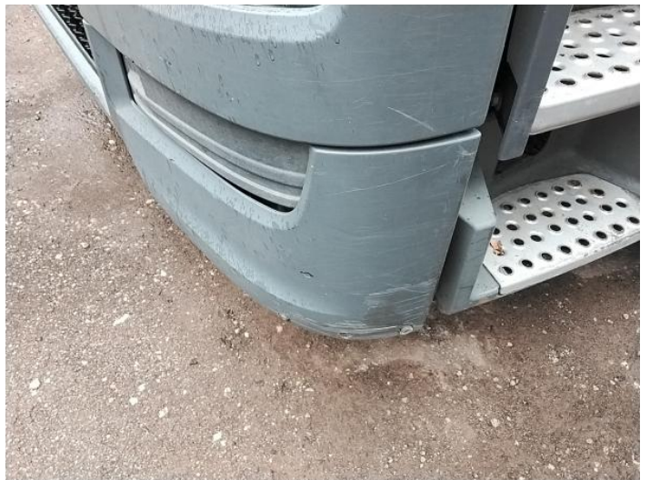
2: Bumper Front Scratched Over 100mm Thru Paint
