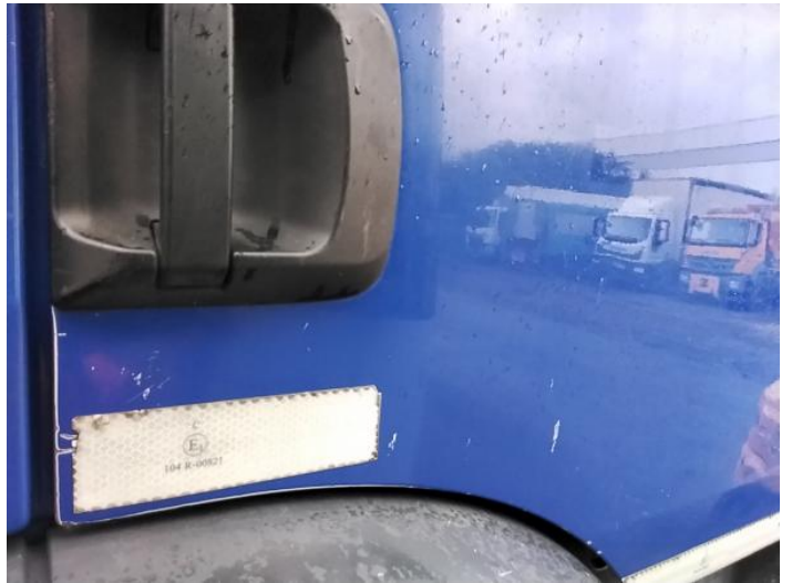
6: Door osf Scratched Over 25mm Thru Paint
