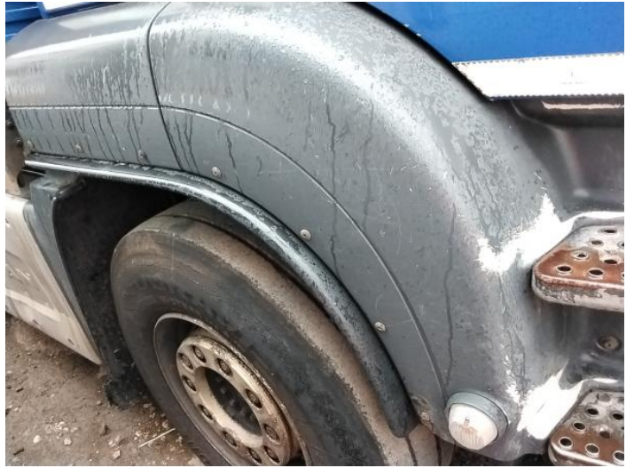
4: Wing osf Scratched Over 25mm Thru Paint
