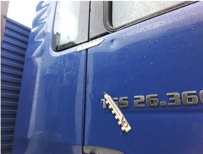
5: Door osf Dented Over 30mm
