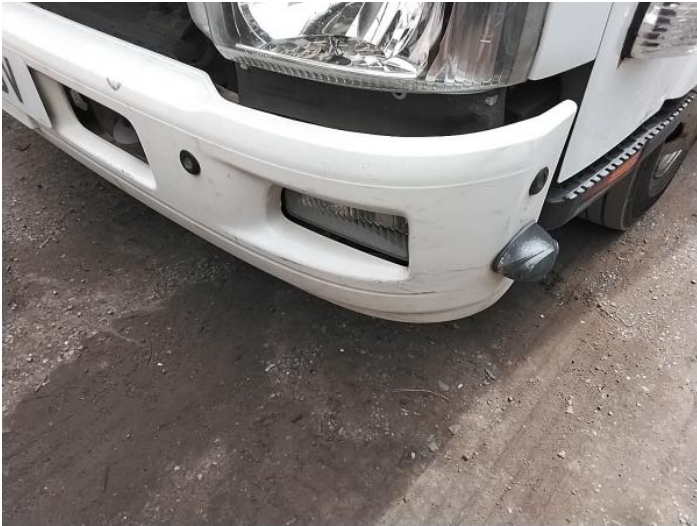
9: Bumper Front Scratched Over 100mm Thru Paint
