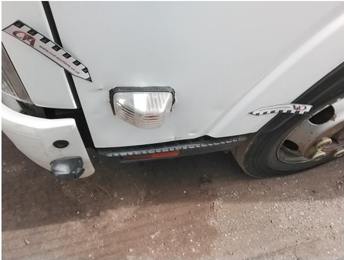
10: Door nsf Dented With Paint Damage
