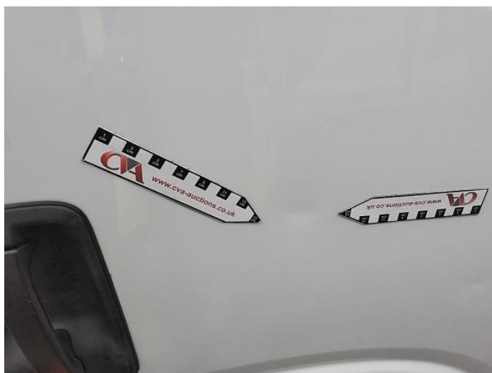
2: Door osf Dented Over 30mm
