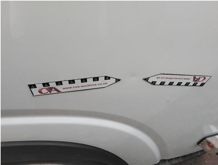
3: Door osf Dented Over 30mm
