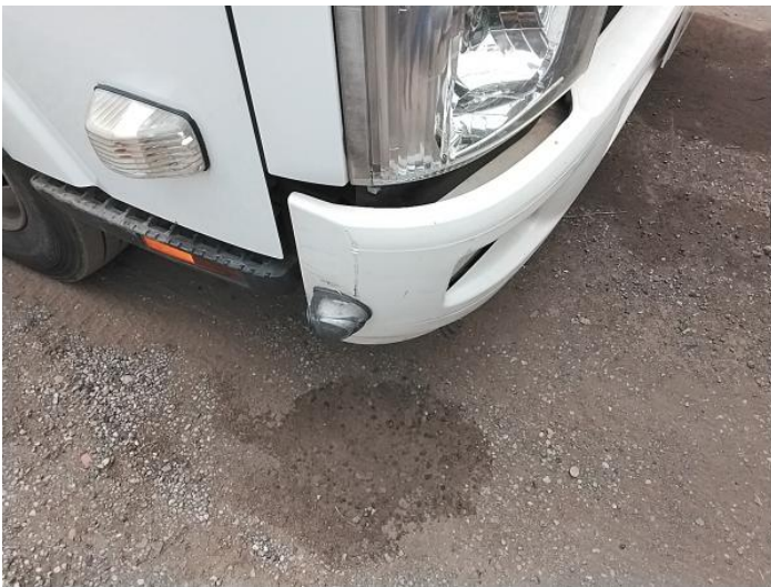
5: Bumper Front Scratched Over 100mm Thru Paint
