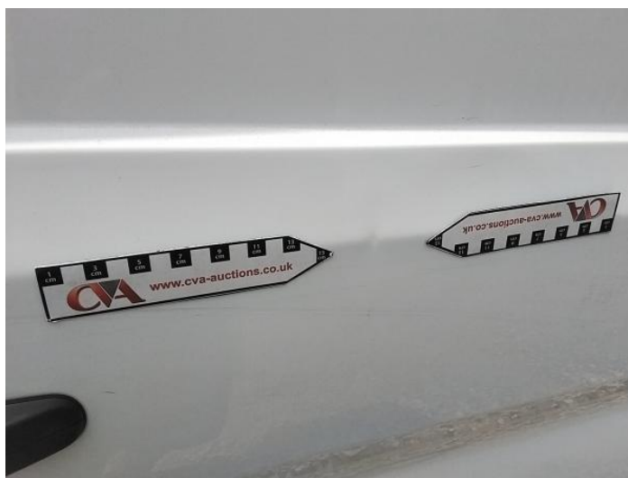
2: Qtr Panel nsr Dented Over 30mm
