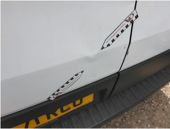
9: Door nsr Dented Over 30mm
