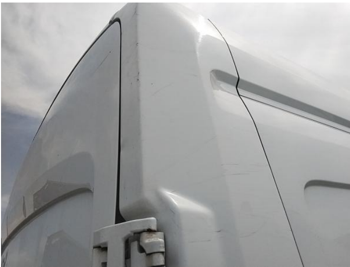
11: C Post os Scratched Over 25mm Thru Paint
