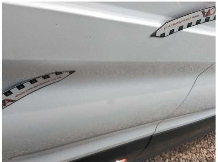
12: Qtr Panel osr Dented Over 30mm
