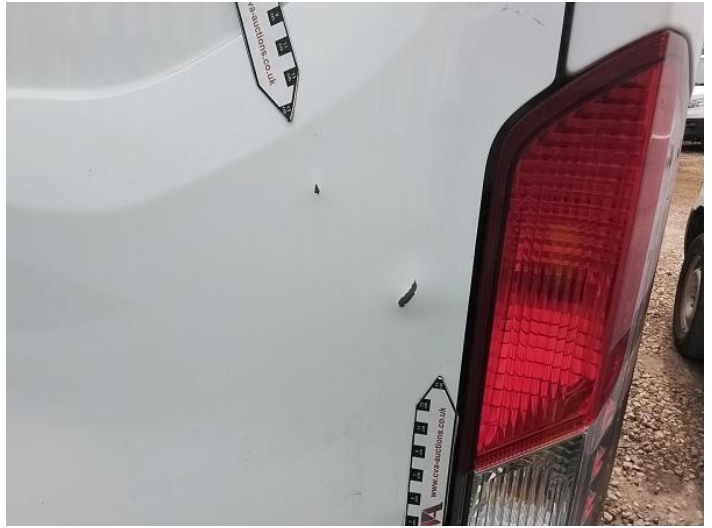
10: Door osr Dented With Paint Damage
