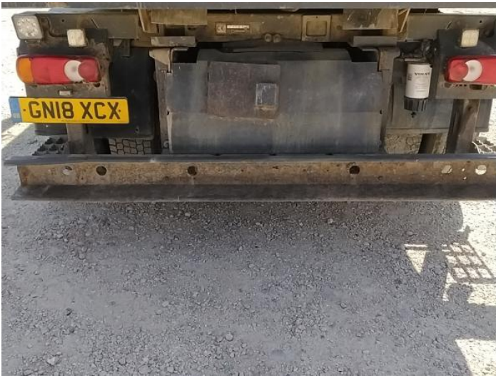
11: Bumper Rear Dented Over 30mm
