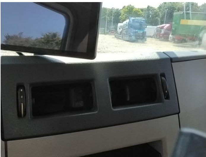
13: Air Vents nsf Missing Replace
