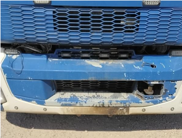
3: Bumper Front Chipped Multiple Chips
