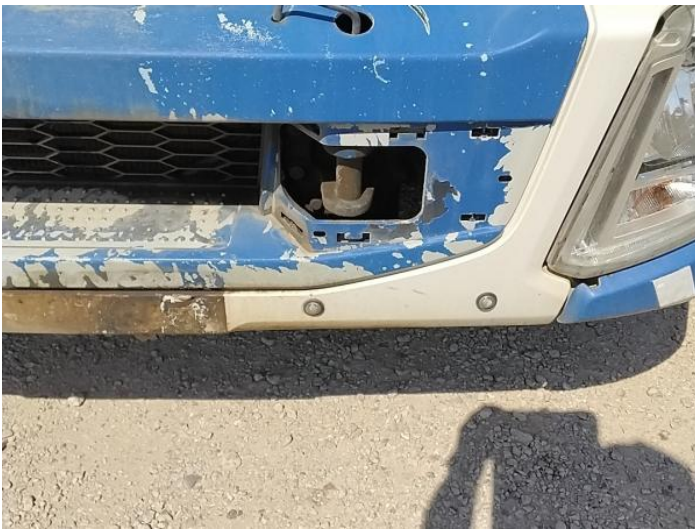
5: Front TowEye Cvr Missing Replace
