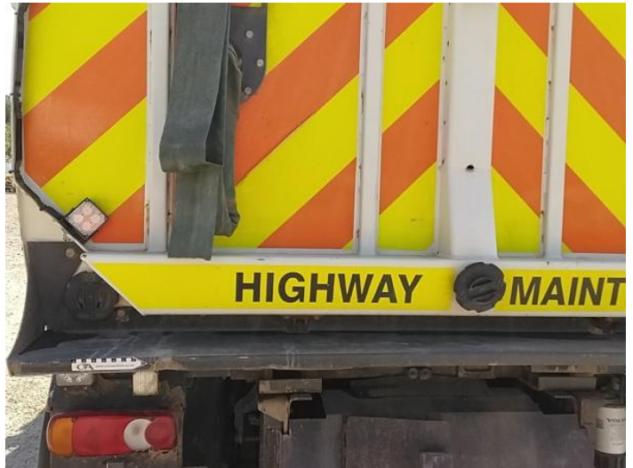
12: Panel Rear Dented With Paint Damage
