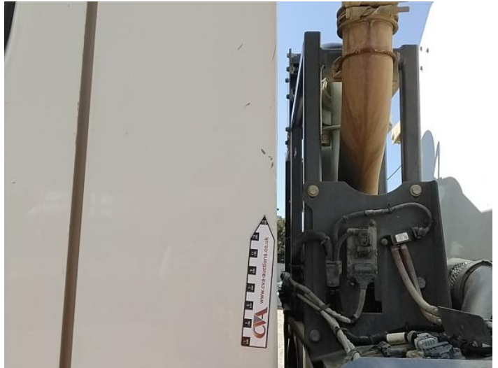
10: B Post ns Dented Over 2 UpTo 10mm
