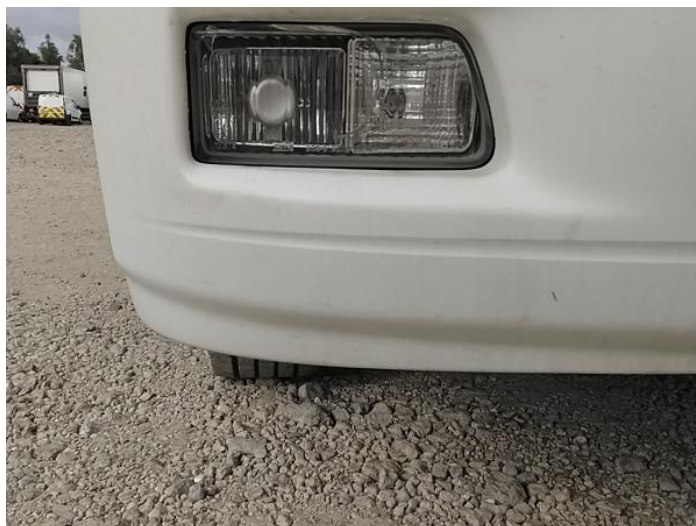
2: Fogdriving Lamp osf Broken Replace
