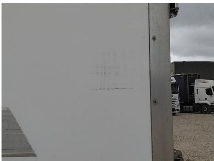
5: Qtr Panel nsr Scratched Over 25mm Not Thru Paint
