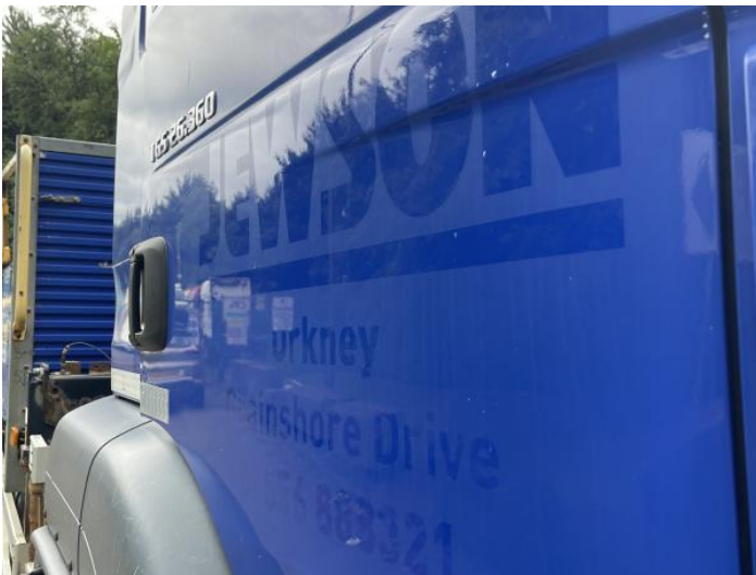
5: Door osf Dented Over 30mm
