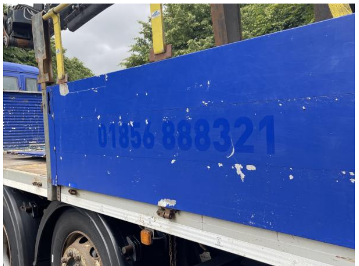
8: Qtr Panel nsr Dented With Paint Damage
