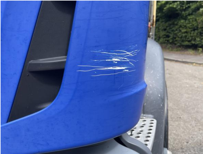
3: Wing nsf Scratched Over 25mm Thru Paint
