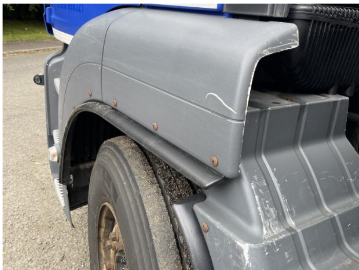
9: Door Moulding nsf Scuffed (Unpainted) Over 100mm
