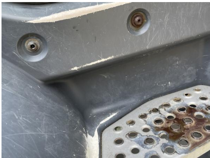
1: Door Moulding of Scuffed (Unpainted) Over 100mm
