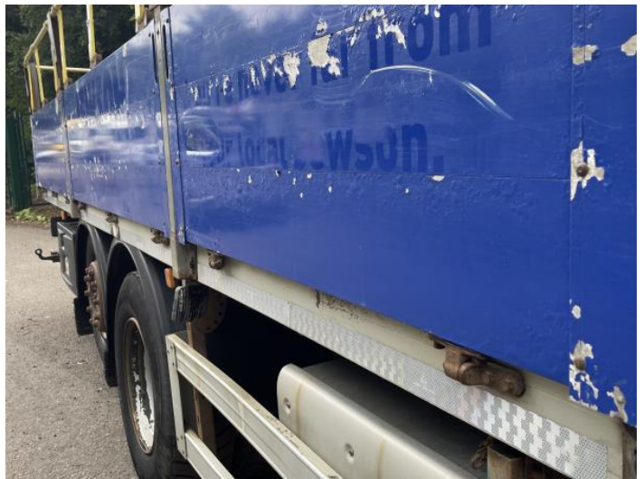
6: Qtr Panel osr Dented Over 30mm
