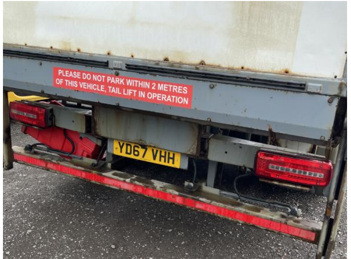
10: Tailgate Rusted Over 5mm
