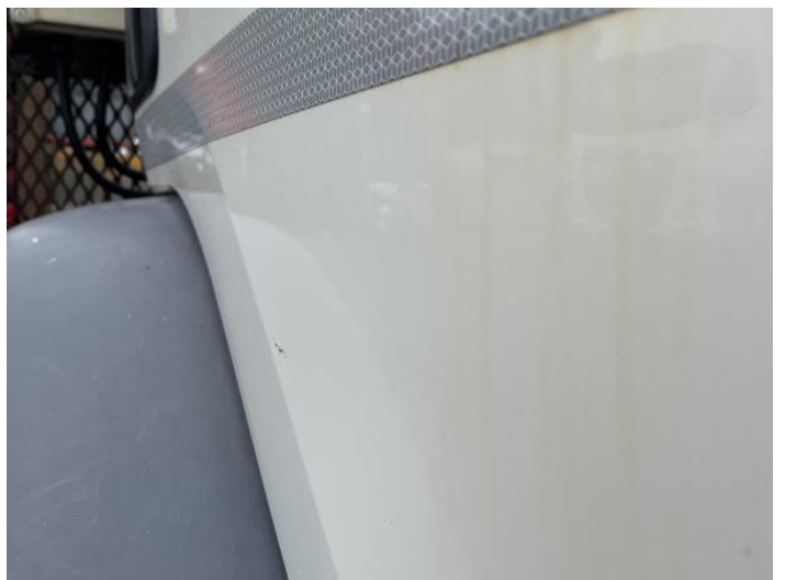
8: Door osf Dented Over 30mm
