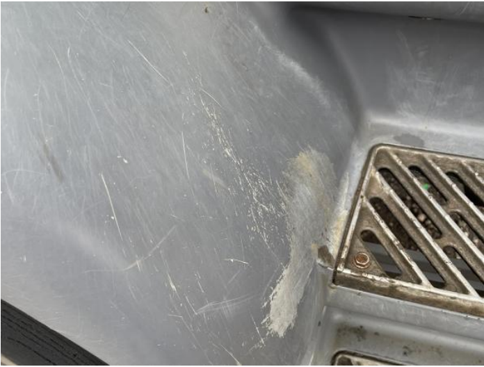
3: Door Moulding osf Scuffed (Unpainted) Over 100mm
