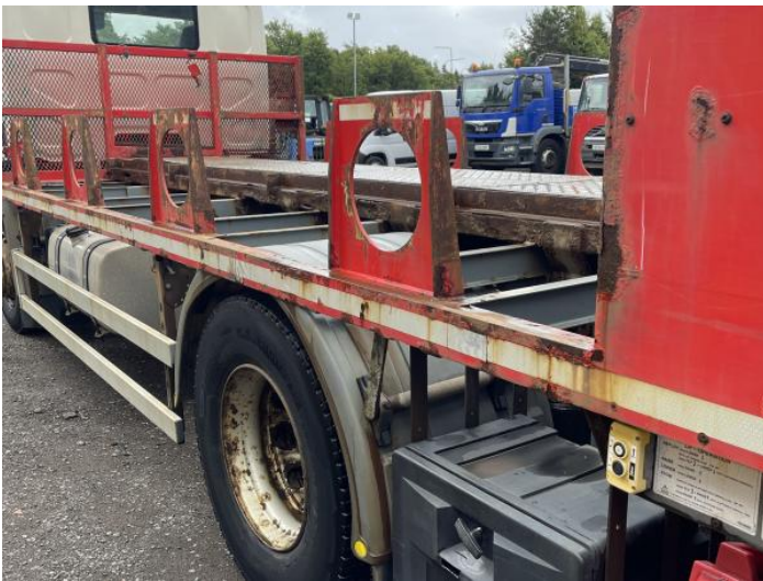
11: Qtr Panel nsr Rusted Over 5mm
