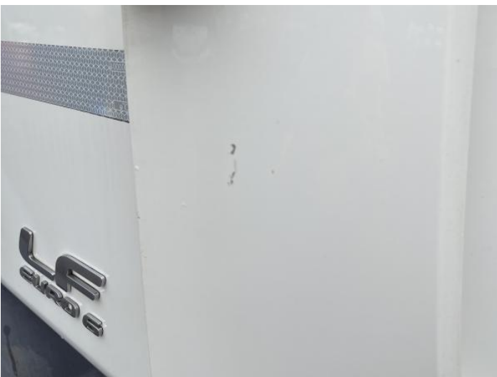
7: Wing osf Scratched UpTo 25mm Thru Paint
