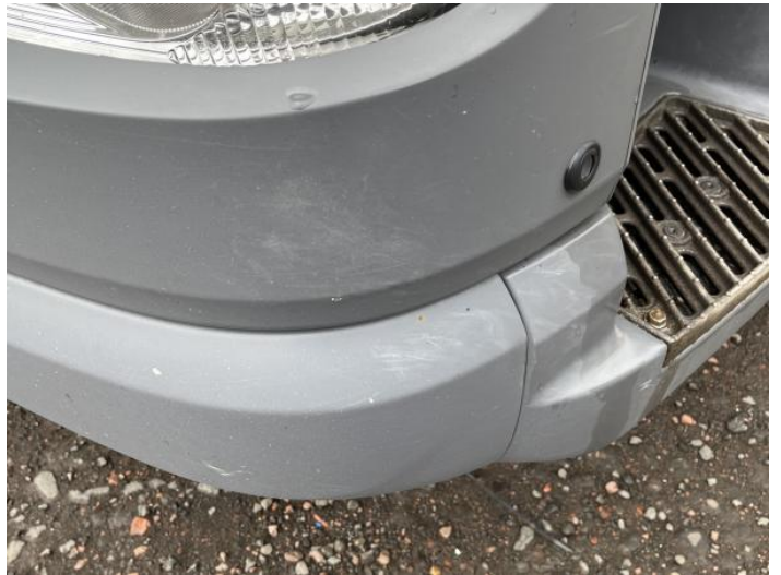
6: Bumper Front Scratched UpTo 25mm Not Thru Paint
