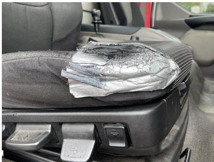
2: Seat Base Cover osf Torn Over 3mm
