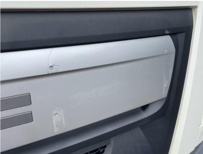
5: Bumper Front Grill Broken Replace
