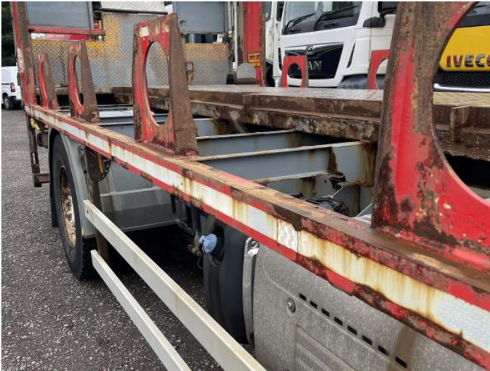
9: Qtr Panel osr Rusted Over 5mm
