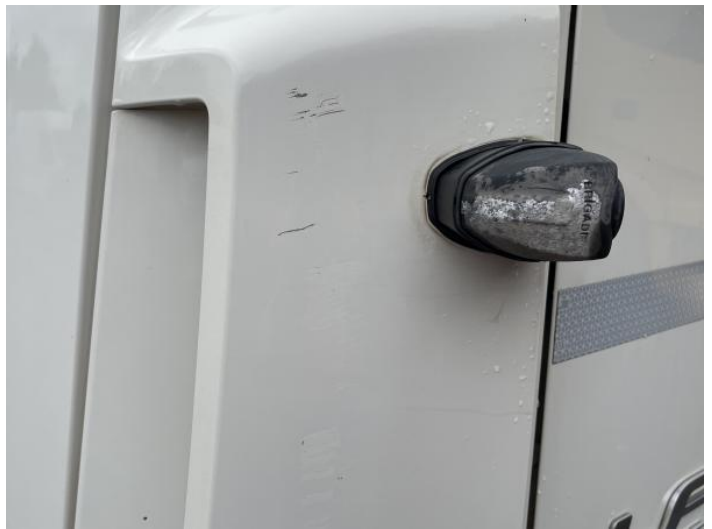
12: Wing nsf Scratched UpTo 25mm Thru Paint
