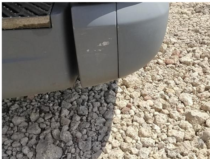
2: Bumper Front Scratched 25 to 100mm Thru Paint
