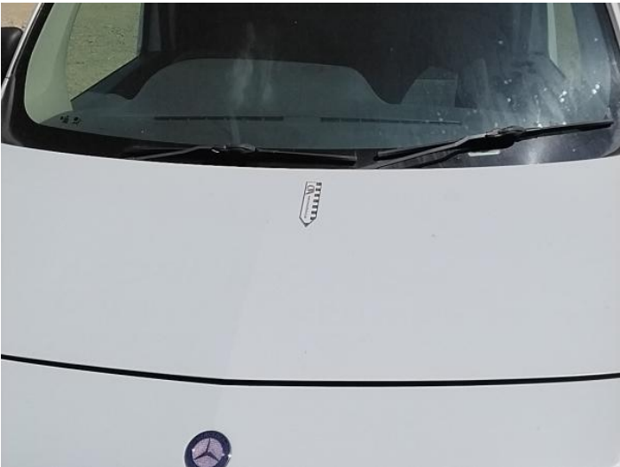
1: Bonnet Chipped Multiple Chips
