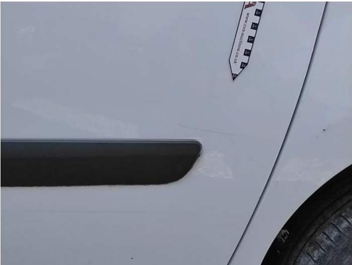
2: Door nsr Scratched Over 25mm Thru Paint
