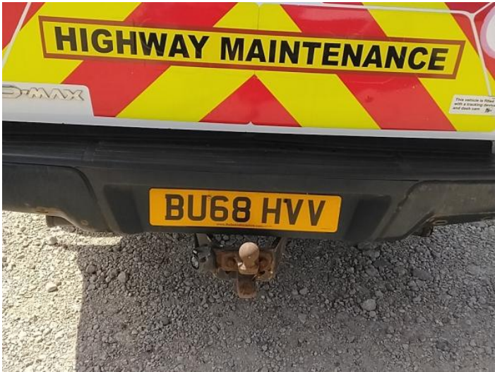
6: Bumper Rear Rusted Over 5mm
