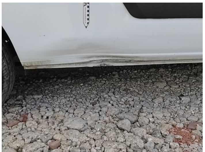
14: Sill os Dented With Paint Damage
