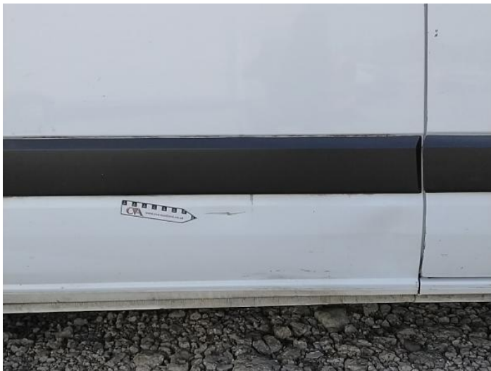
15: Qtr Panel osr Dented With Paint Damage
