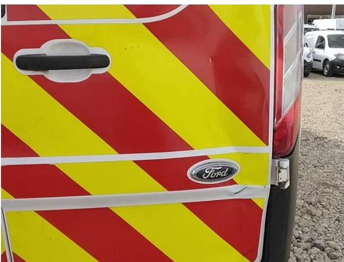
13: Door osr Dented With Paint Damage
