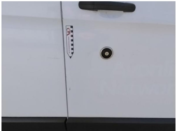
16: Door osf Dented Over 2 UpTo 10mm
