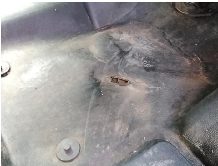
17: Carpets Front Holed Over 3mm
