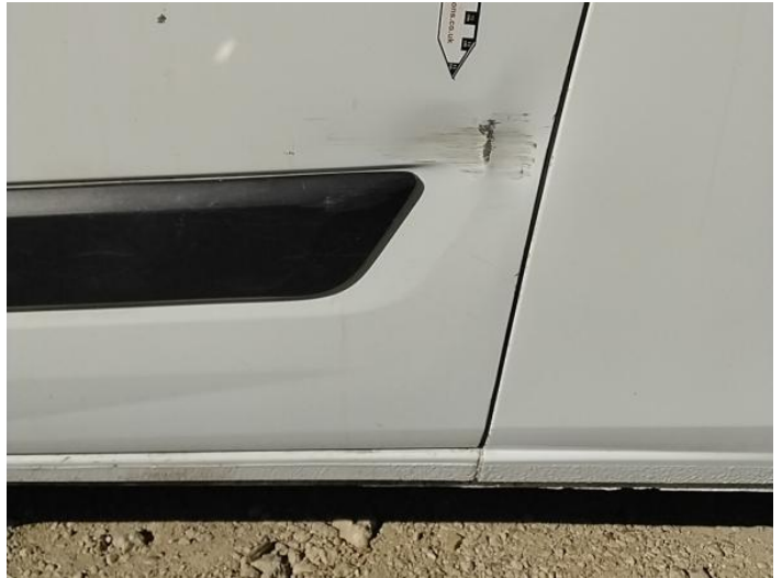
10: Door nsr Dented With Paint Damage
