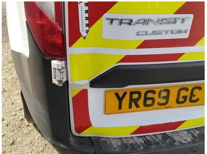
12: Door nsr Dented With Paint Damage
