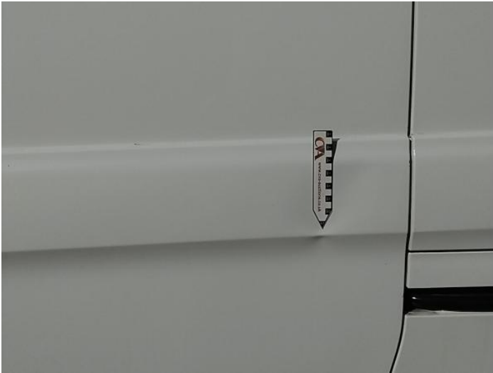
9: Door nsr Dented 2 Or Less UpTo 10mm
