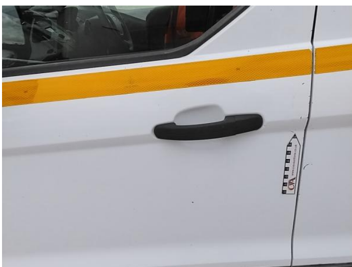
7: Door nsf Dented Between 10mm + 30mm
