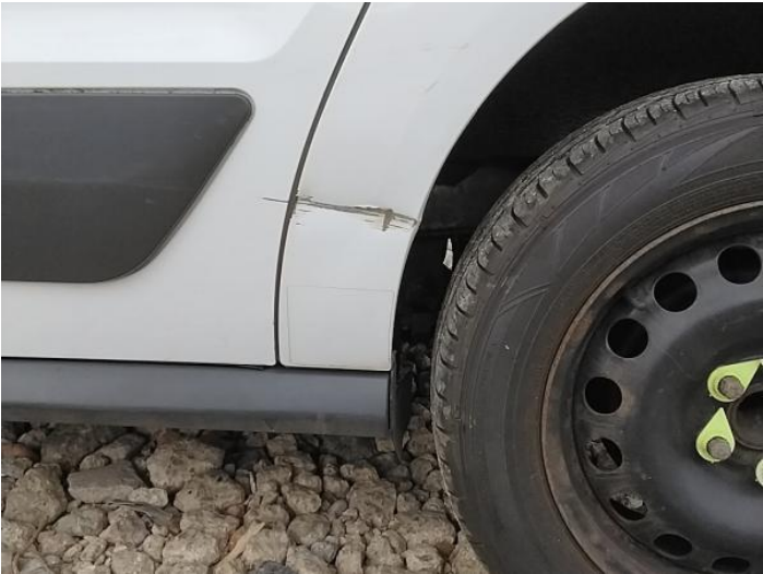
10: Qtr Panel nsr Dented With Paint Damage
