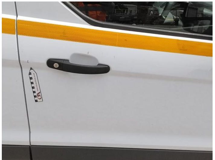
18: Door osf Dented 2 Or Less UpTo 10mm
