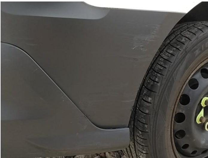
17: Qtr Panel Moulding os Scuffed (Unpainted) Over 100mm
