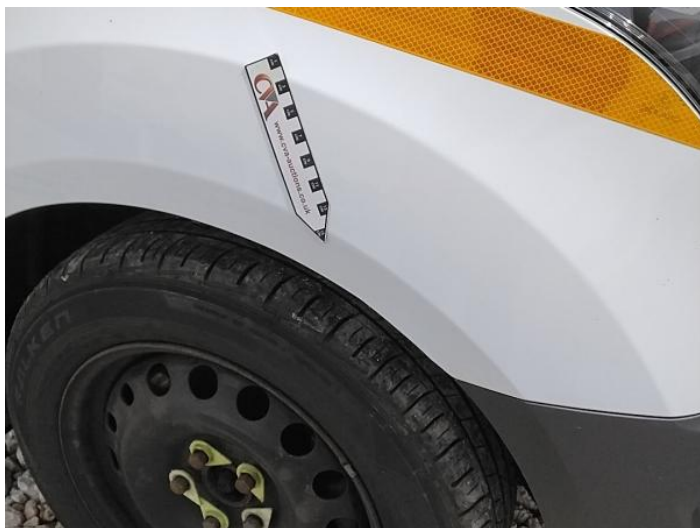
1: Wing of Dented Over 30mm
