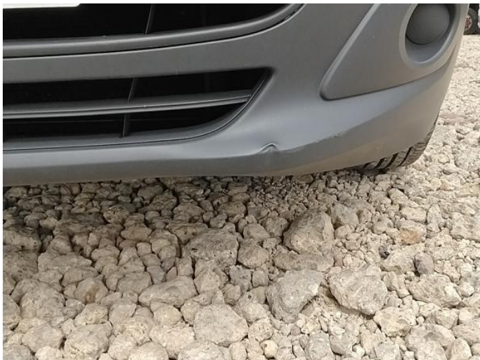
3: Bumper Front Dented Between 10mm + 30mm
