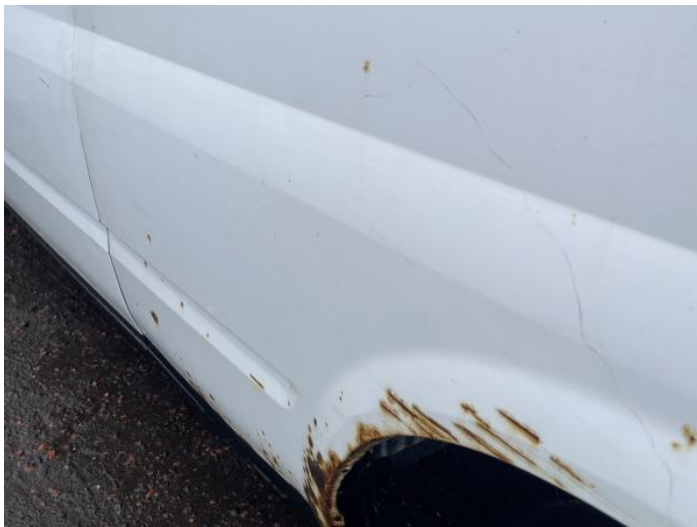
11: Qtr Panel nsr Rusted Over 5mm
