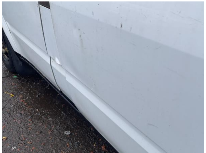
12: Door nsr Dented Over 30mm
