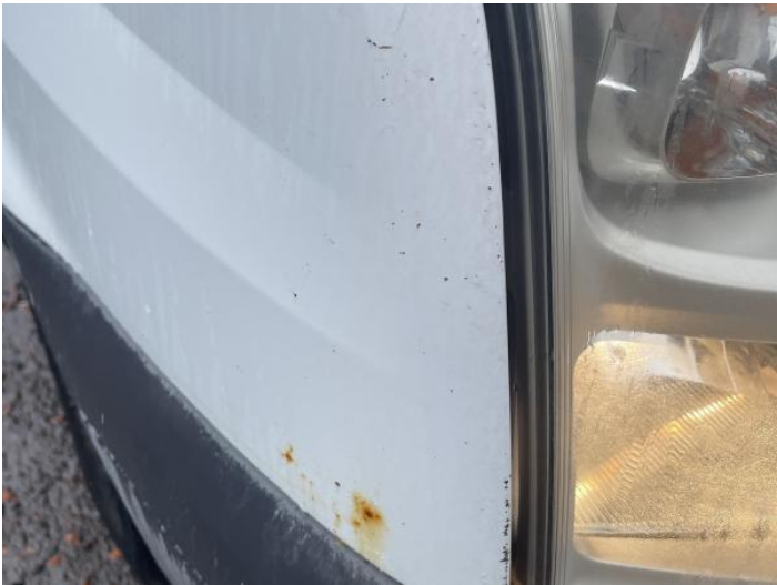
5: Wing of Rusted Over 5mm
