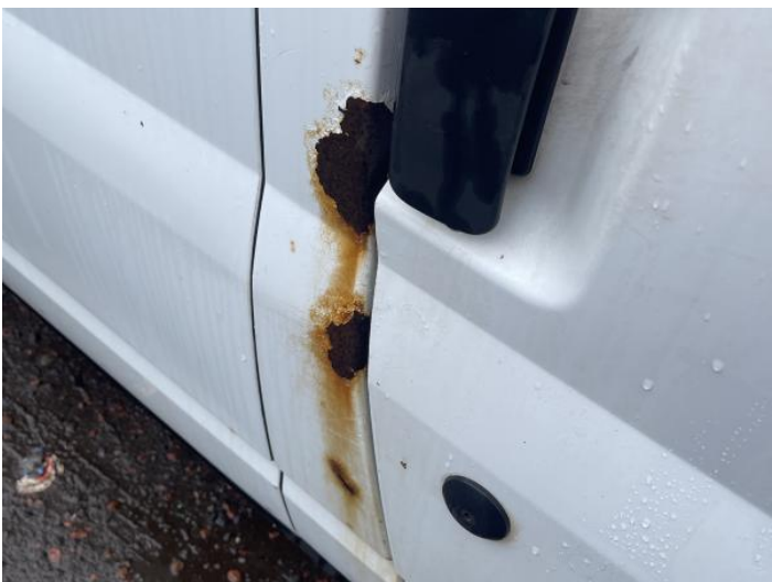
7: B Post os Rusted Over 5mm
