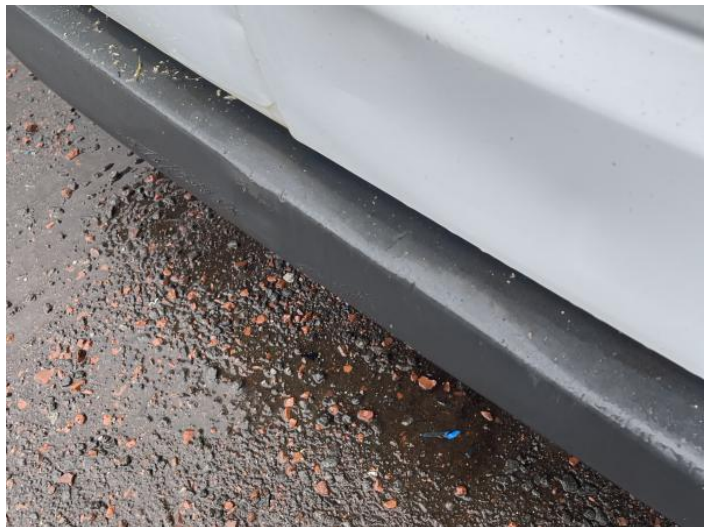
10: Bumper Rear Moulding Scuffed (Unpainted) Over 100mm
