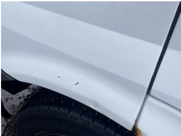
15: Wing nsf Dented With Paint Damage
