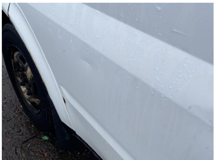
14: Door nsf Dented Over 30mm
