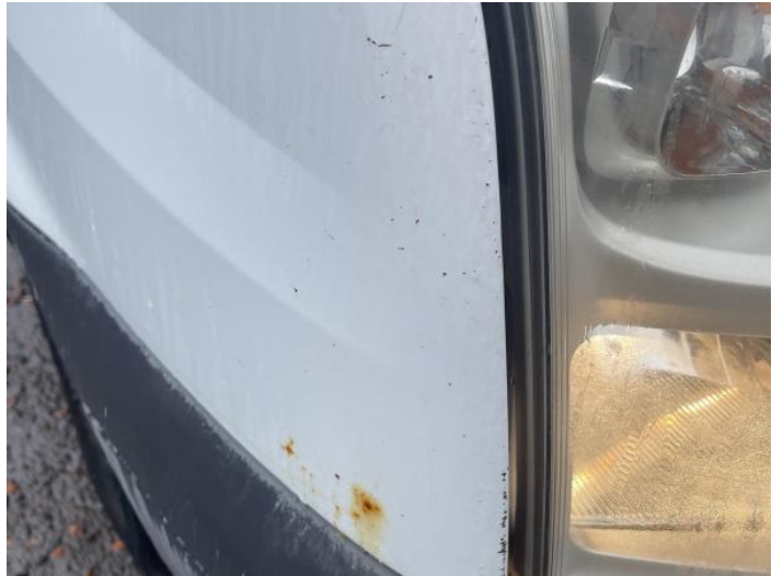
4: Wing osf Rusted Over 5mm
