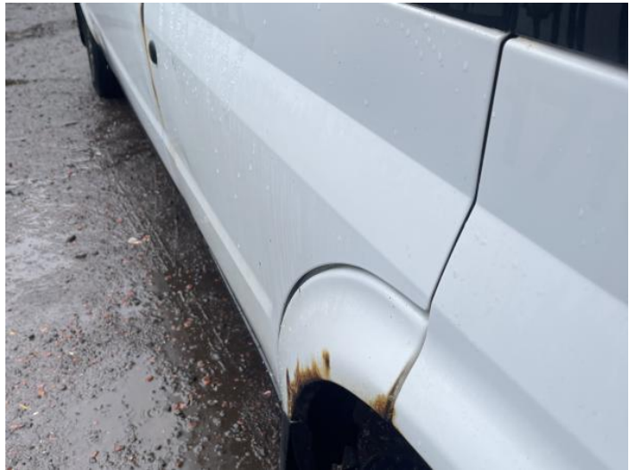
6: Door osf Rusted Over 5mm
