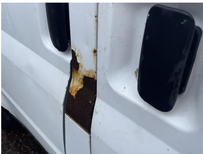
13: B Post ns Rusted Over 5mm
