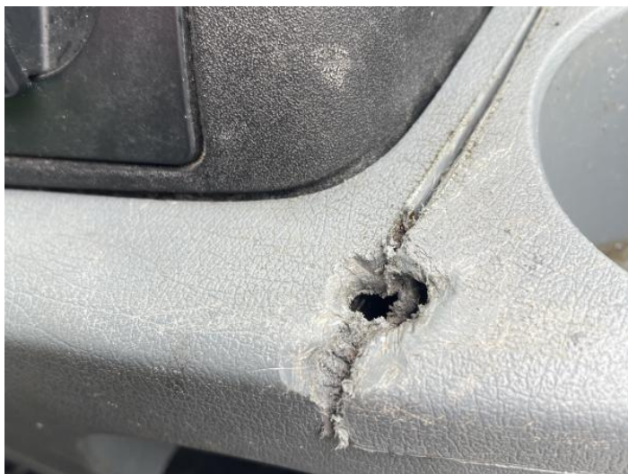
1: Centre Console Front Holed Over 3mm
