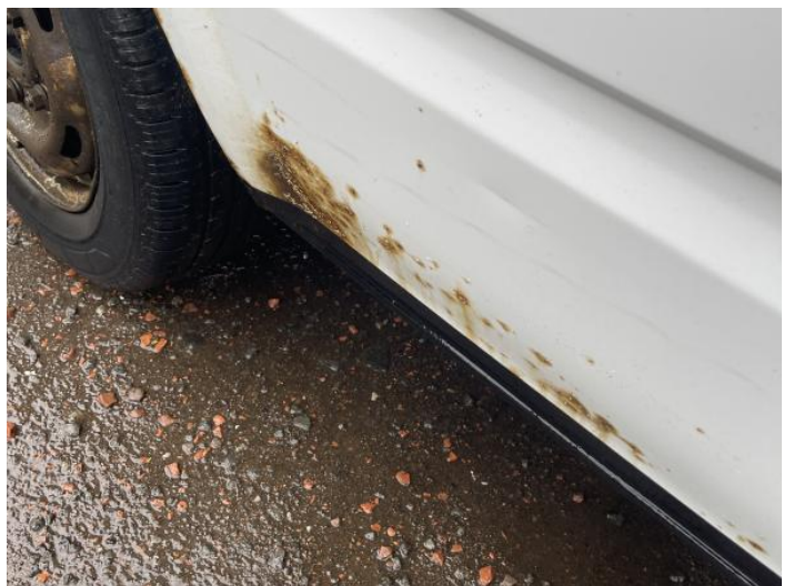
8: Qtr Panel osr Rusted Over 5mm
