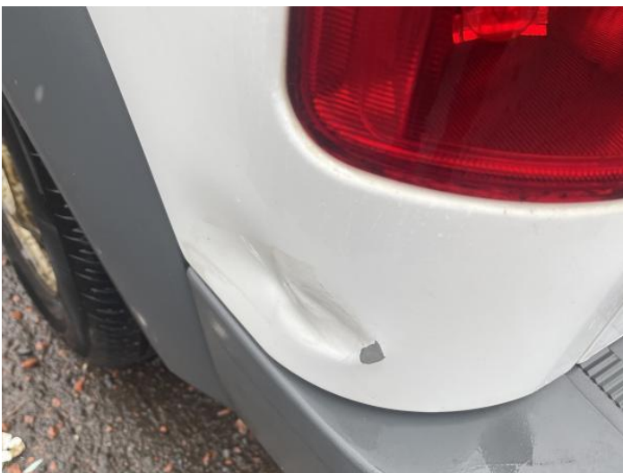
7: Qtr Panel nsr Dented Over 30mm
