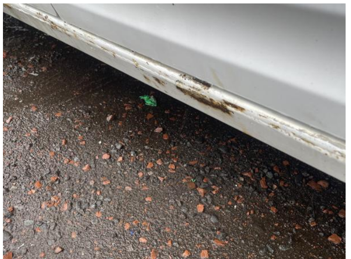
8: Sill ns Dented Over 30mm
