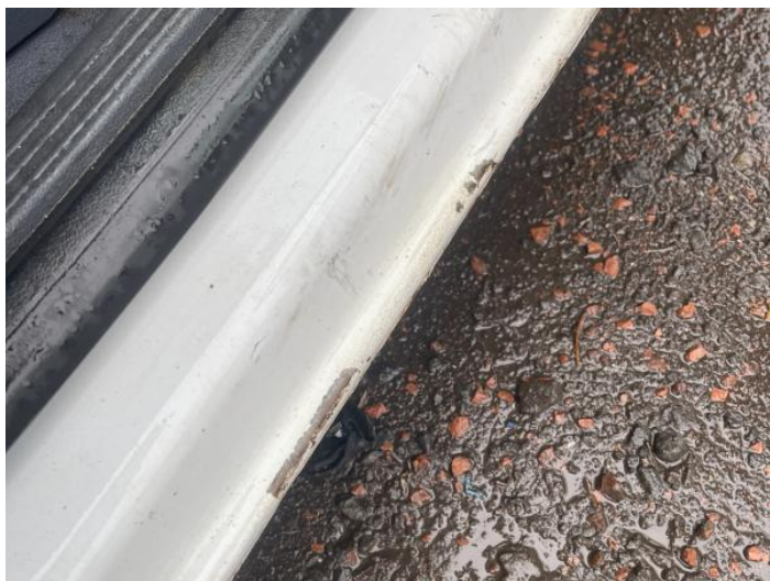
1: Sill os Rusted Over 5mm
