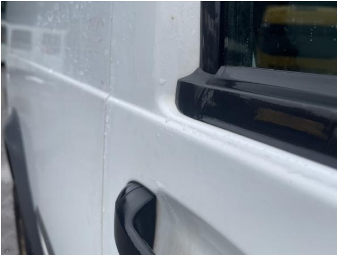
3: Door osf Dented Between 10mm + 30mm
