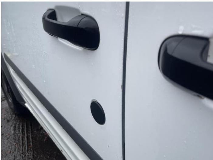
9: Door nsf Dented Between 10mm + 30mm
