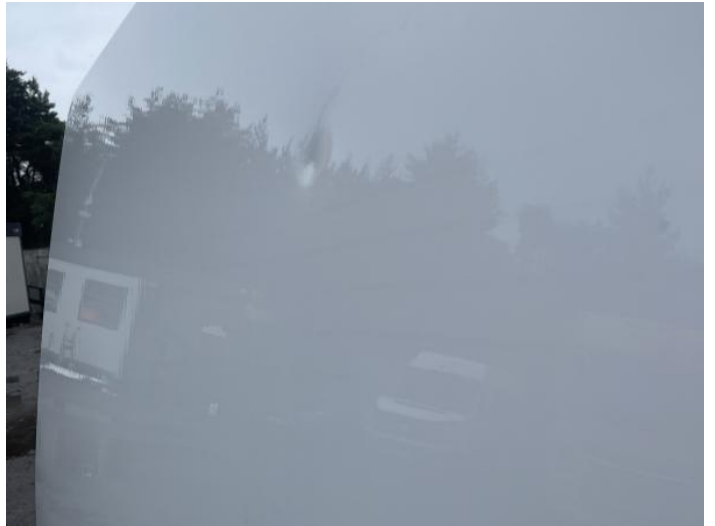
4: Qtr Panel osr Dented Between 10mm + 30mm
