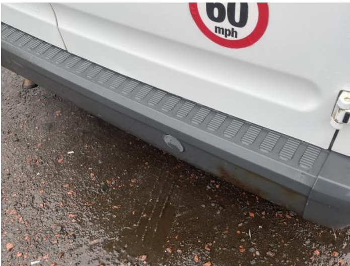
5: Bumper Rear Moulding Scuffed (Unpainted) UpTo 100mm
