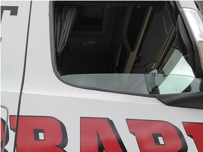
21: Door osf Scratched Over 25mm Thru Paint
