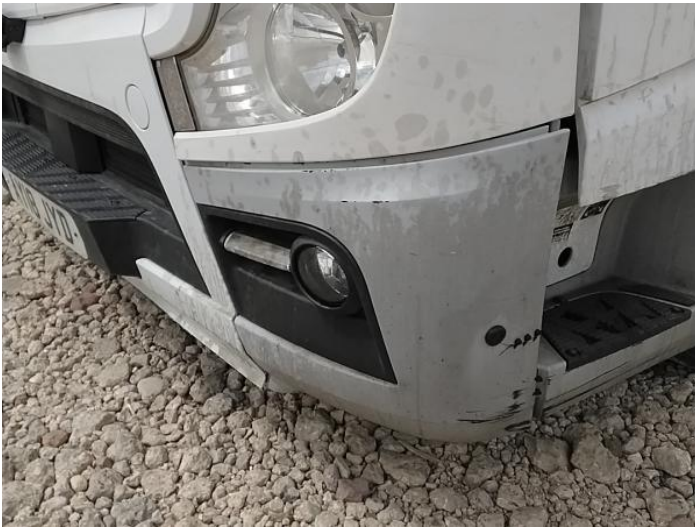
5: Bumper Front Poor Previous Repair Poor Paint
