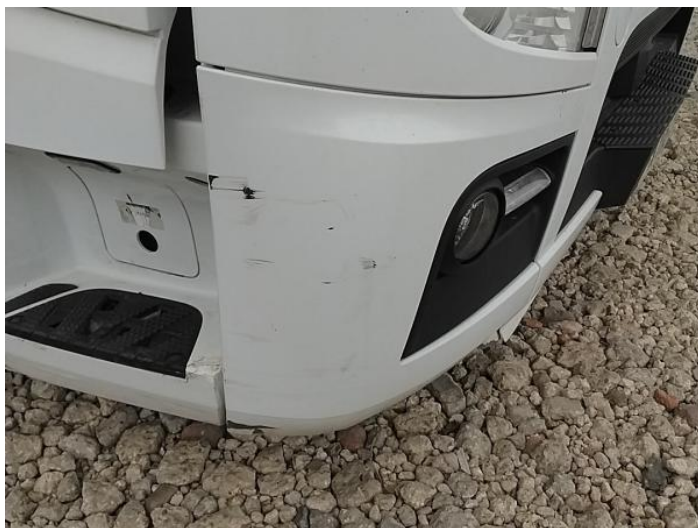
1: Bumper Front Scratched Over 100mm Thru Paint
