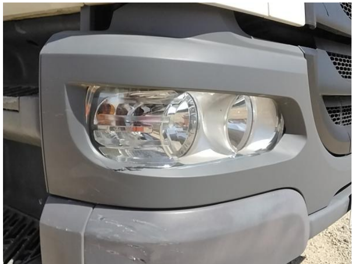
2: Fog Lamp Surround is Broken Replace
