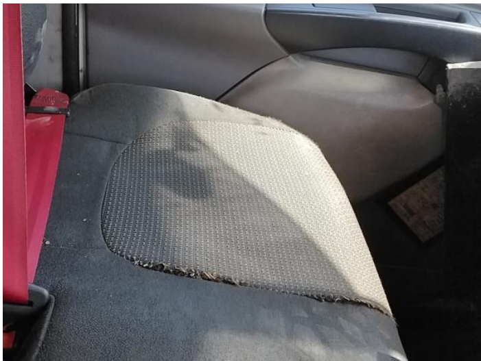
15: Seat Base Cover nsf Scuffed Over 25mm
