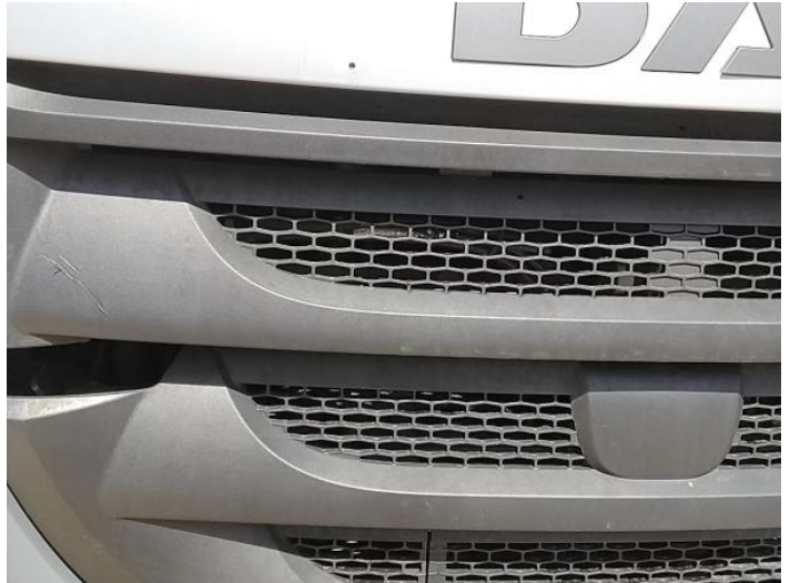
4: Grille Front Scuffed (Unpainted) UpTo 100mm
