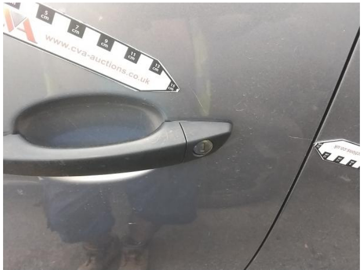
6: Door nsf Scratched Over 25mm Thru Paint
