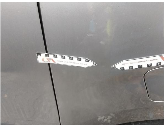
7: Qtr Panel nsr Dented Over 30mm
