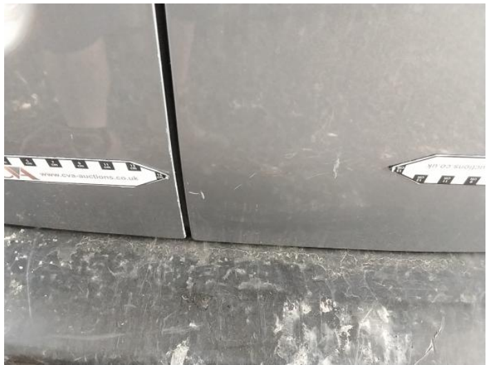
12: Door osr Scratched Over 25mm Thru Paint
