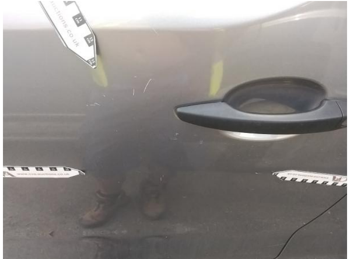
4: Door nsf Scratched Over 25mm Thru Paint
