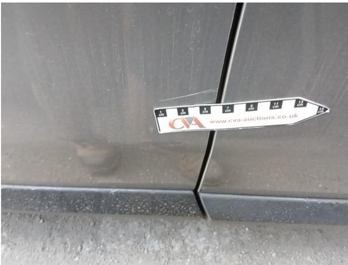
5: Door nsf Scratched Over 25mm Thru Paint
