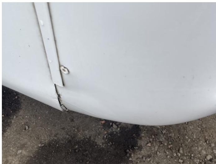
2: Bumper Front Dented With Paint Damage
