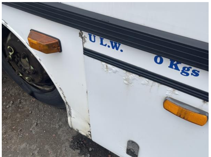
8: Wing nsf Dented With Paint Damage
