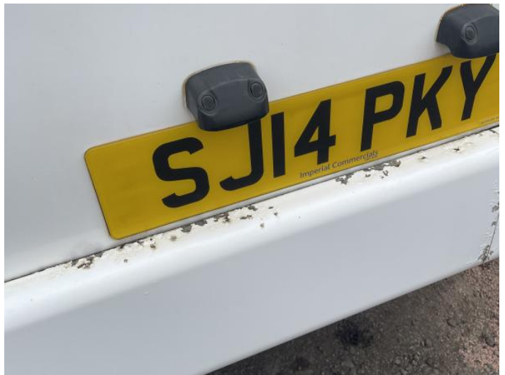
6: Bumper Rear Rusted Over 5mm
