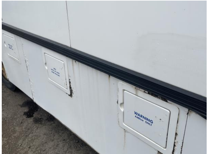
4: Qtr Panel osr Rusted Over 5mm
