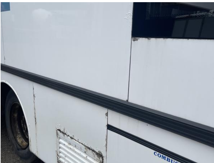
7: Qtr Panel nsr Rusted Over 5mm
