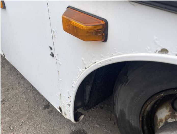
3: Wing osf Rusted Over 5mm
