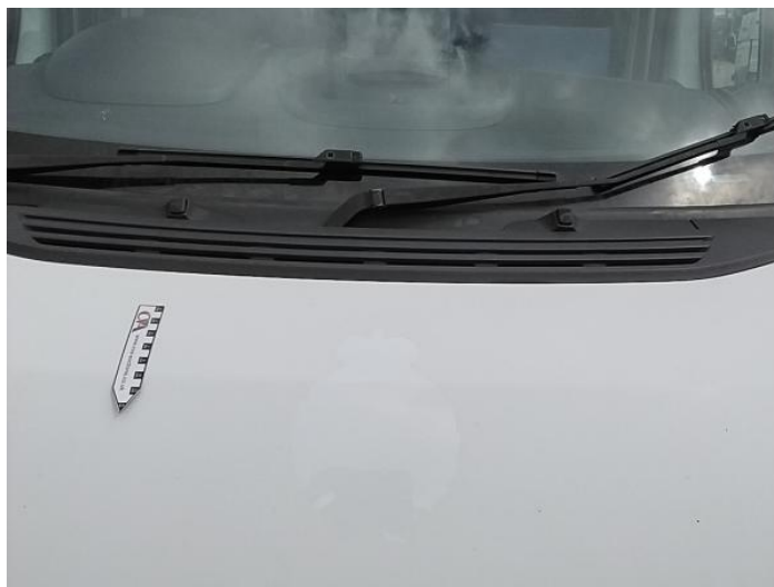
2: Bonnet Chipped Multiple Chips
