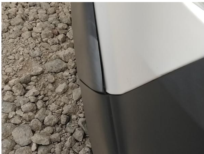
1: Wing Front Arch Extension os Broken Replace
