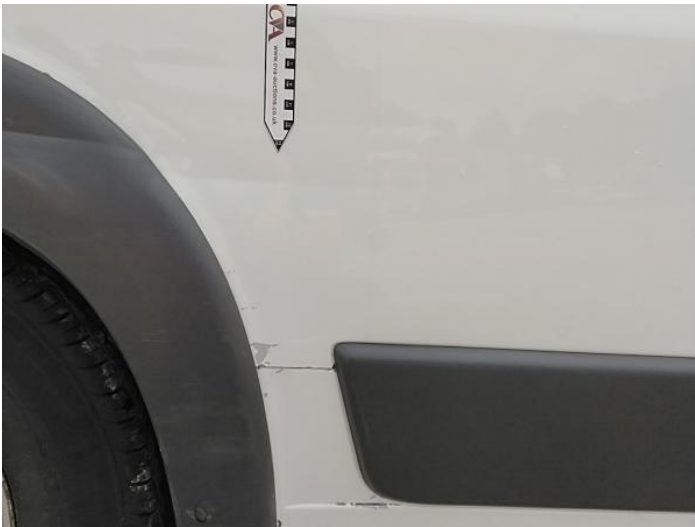
7: Qtr Panel osr Dented With Paint Damage
