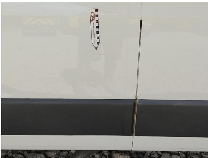
11: Qtr Panel osr Dented With Paint Damage
