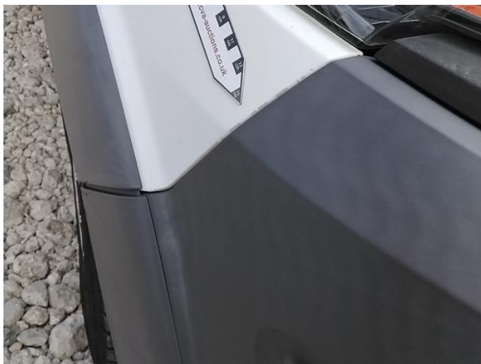
1: Wing osf Chipped Edge Chip
