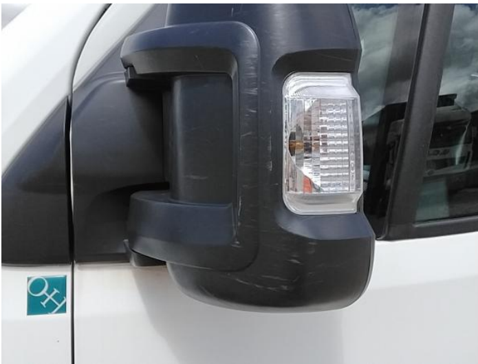
5: Door Mirror Assy nsf Scuffed (Unpainted) Over 100mm
