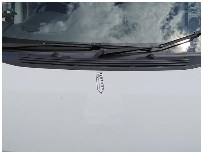
2: Bonnet Chipped Multiple Chips
