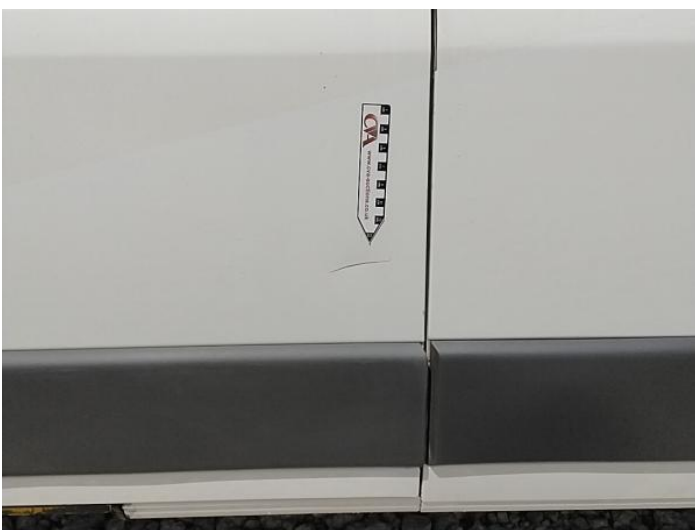
7: Door nsr Dented With Paint Damage
