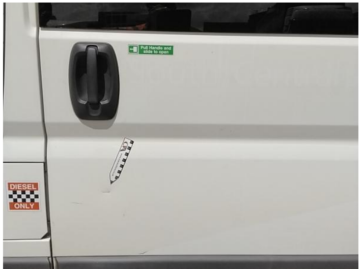
6: Door nsr Dented With Paint Damage
