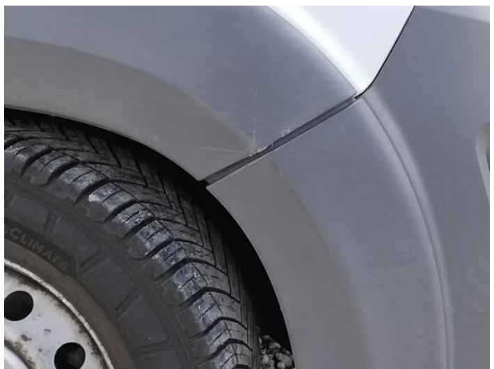
12: Moulding osf Wing Scuffed (Unpainted) UpTo 100mm
