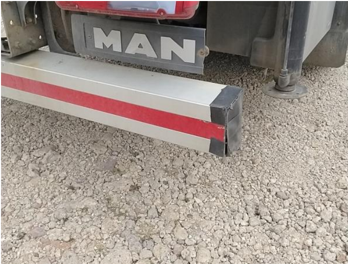
3: Bumper Rear Missing Replace
