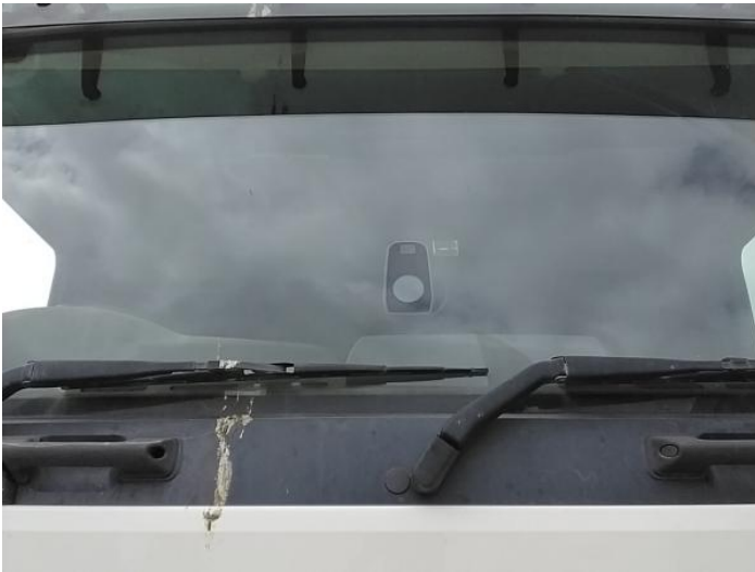
5: Screen Front Chipped Over 10mm
