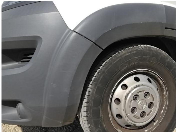
6: Moulding nsf Wing Scuffed (Unpainted) Over 100mm
