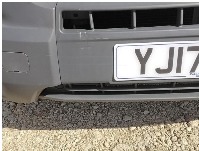
2: Bumper Front Dented Between 10mm + 30mm
