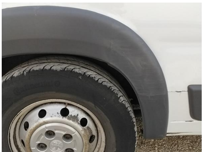
8: Qtr Panel Arch Extension os Scuffed (Unpainted) Over 100mm
