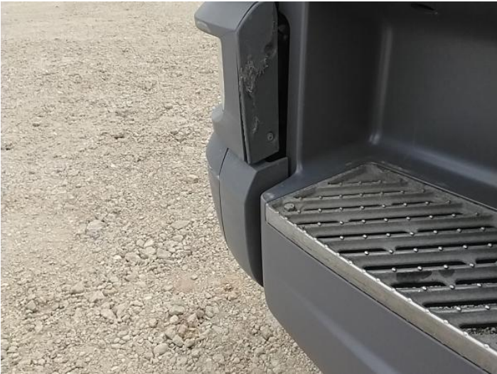
4: Fog Lamp Surround ns Broken Replace
