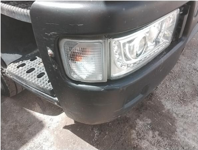
3: Bumper Front Scratched Over 100mm Thru Paint
