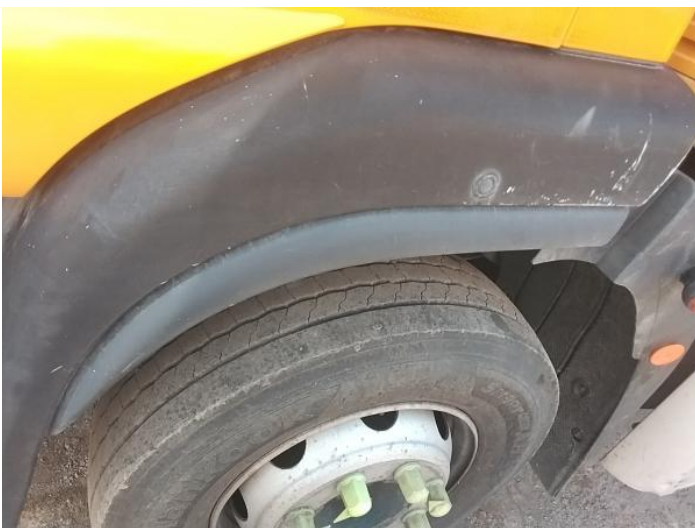
7: Wing nsf Scratched Over 25mm Thru Paint
