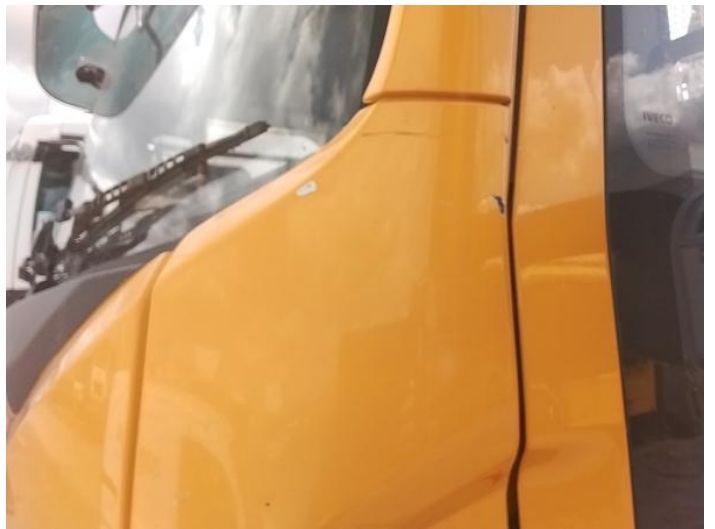
6: Panel Front Scratched Over 25mm Thru Paint
