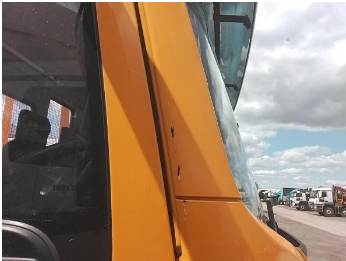
1: A Post os Scratched Over 25mm Thru Paint
