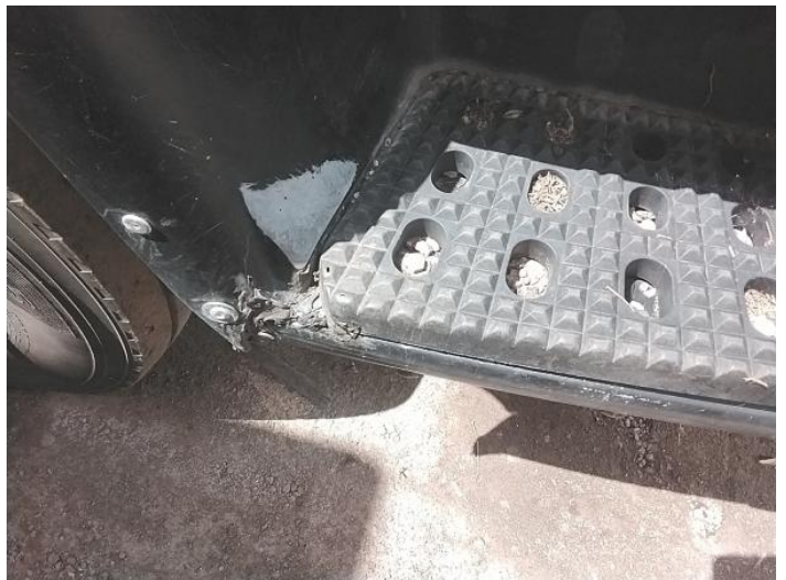
2: Bumper Front Moulding Broken Replace
