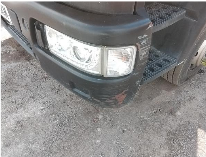
5: Bumper Front Scratched Over 100mm Thru Paint
