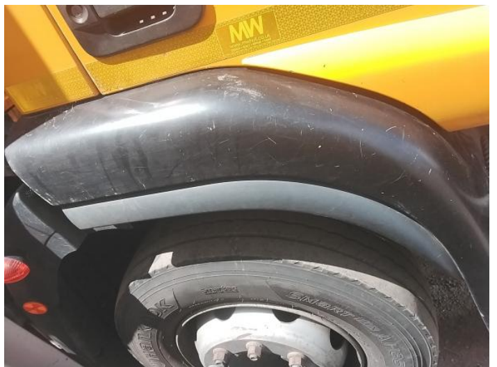
8: Wing osf Scratched Over 25mm Thru Paint
