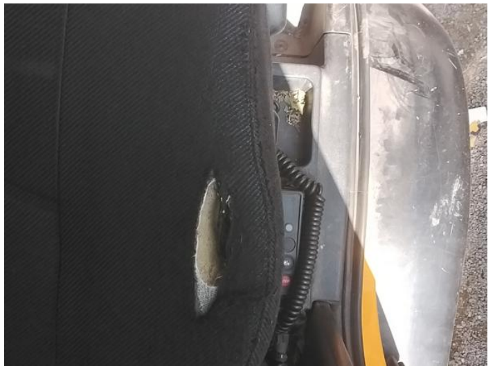
12: Seat Base Cover osf Holed Over 3mm
