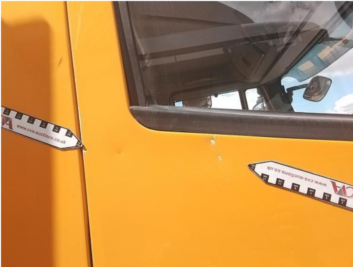
9: Door osf Dented With Paint Damage
