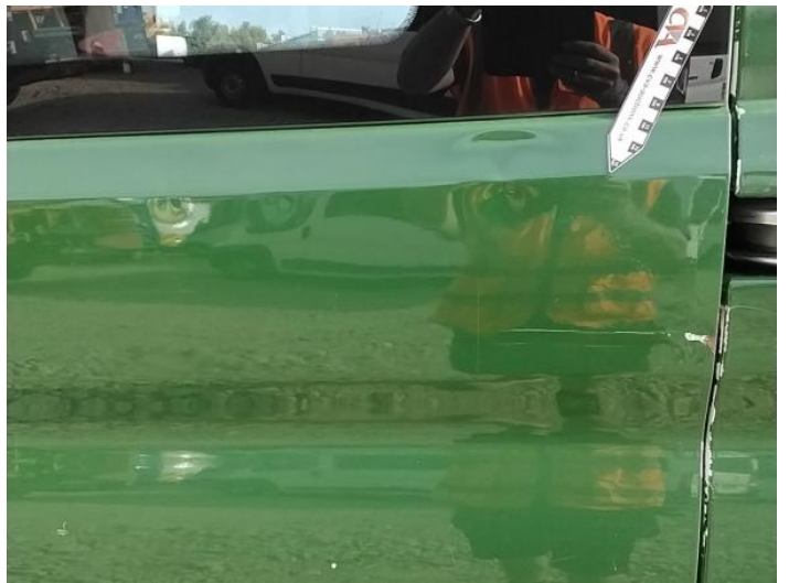
6: Door nsr Dented With Paint Damage
