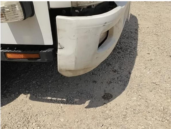
1: Bumper Front Dented Between 10mm + 30mm
