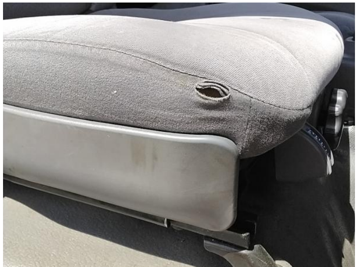
18: Seat Base Cover osf Holed Over 3mm
