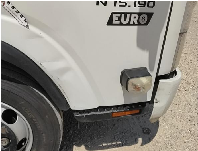
17: Door osf Dented With Paint Damage
