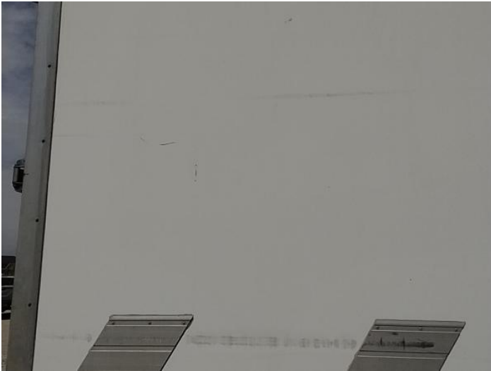
15: Qtr Panel osr Scratched Over 25mm Not Thru Paint
