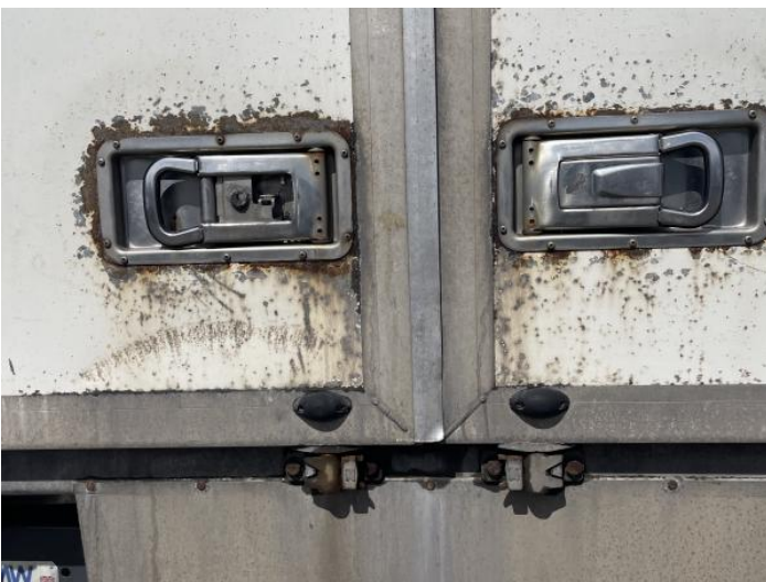
7: Tailgate Rusted Over 5mm
