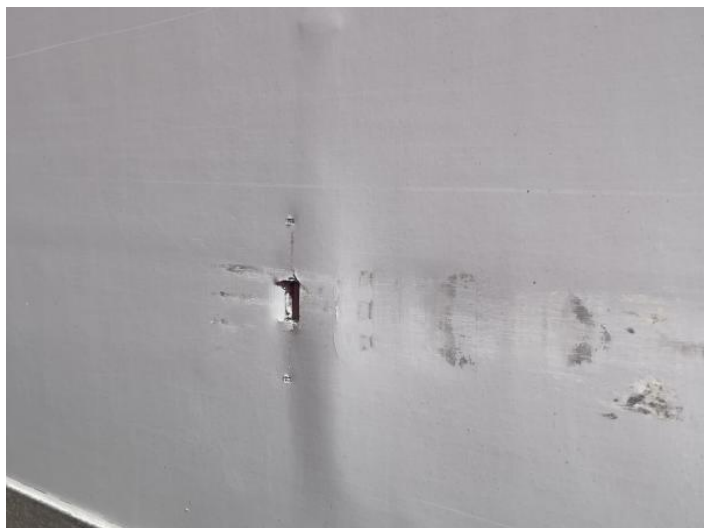
8: Qtr Panel nsr Hole UpTo 10mm
