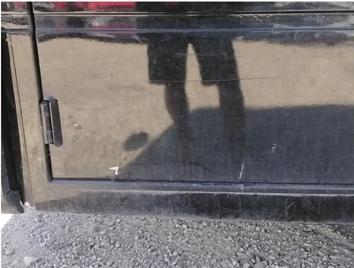
5: Door nsf Scratched UpTo 25mm Thru Paint
