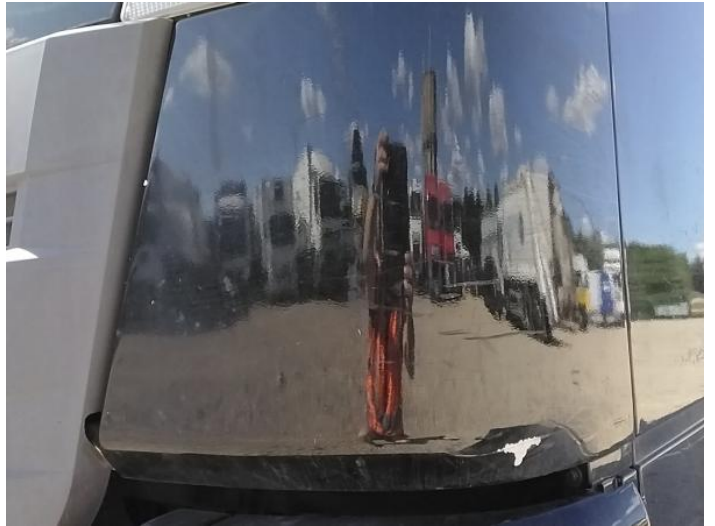
4: Wing nsf Scratched UpTo 25mm Thru Paint
