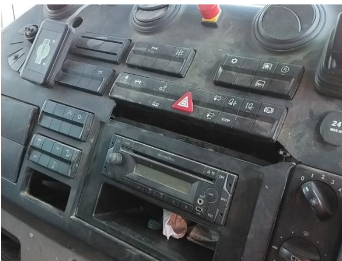
13: Fascia Panel Broken Replace
