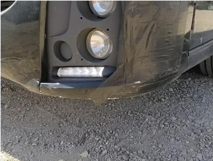
3: Fog Lamp Surround ns Broken Replace
