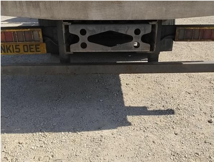
9: Bumper Rear Rusted Over 5mm
