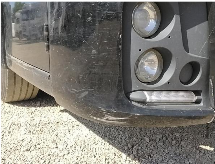
1: Fog Lamp Surround os Scratched (Painted) Over 25mm Thru Paint
