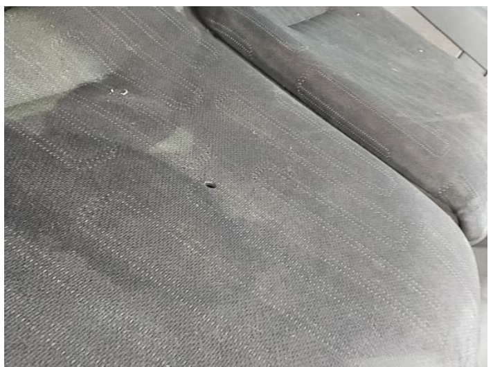
14: Seat Base Cover nsf Burn Over 3mm
