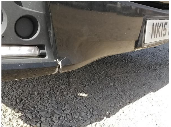
2: Bumper Front Cracked UpTo 25mm
