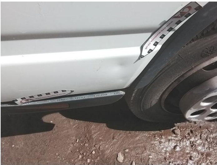
5: Door nsf Dented With Paint Damage
