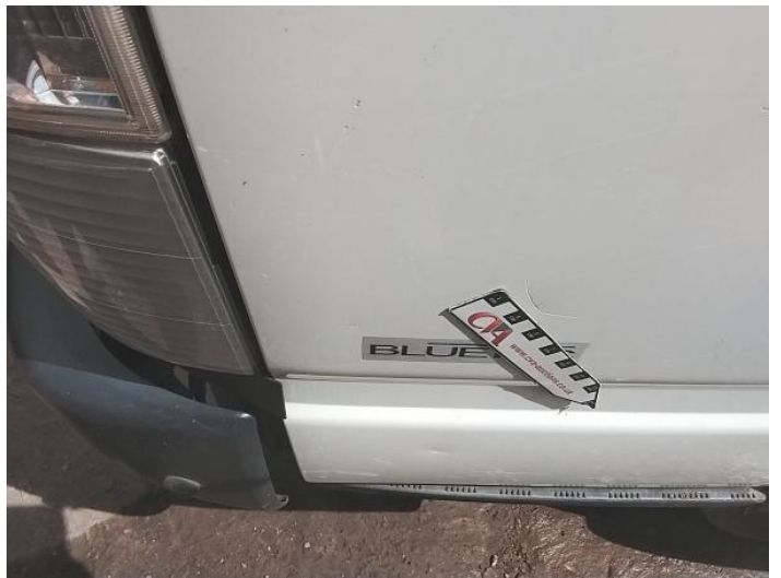
6: Door nsf Scratched Over 25mm Thru Paint
