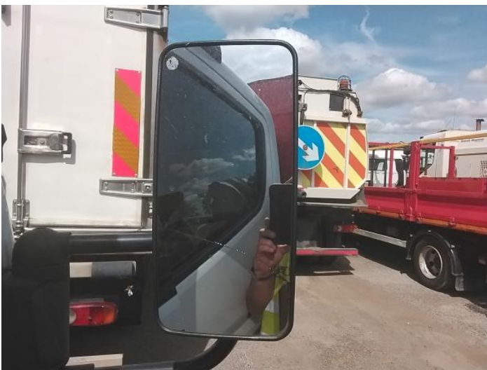
7: Door Mirror Glass os Broken Replace
