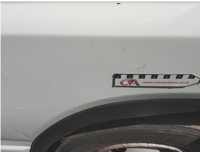
5: Door nsf Scratched Over 25mm Thru Paint
