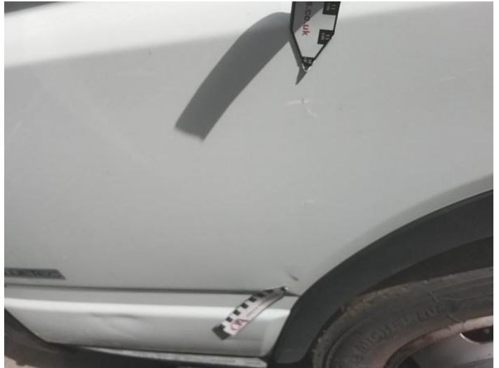
4: Door nsf Scratched Over 25mm Thru Paint
