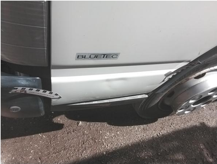
3: Door nsf Dented With Paint Damage
