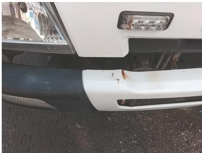
2: Bumper Front Dented With Paint Damage
