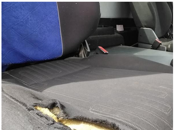
14: Seat Base Cover osf Holed Over 3mm
