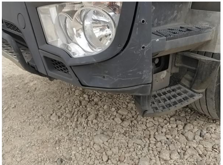
6: Bumper Front Dented Between 10mm + 30mm
