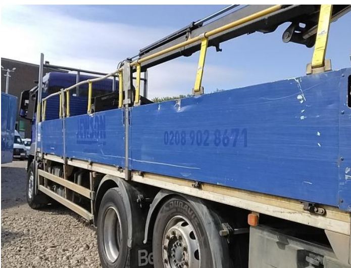
13: Qtr Panel nsr Dented Over 30mm
