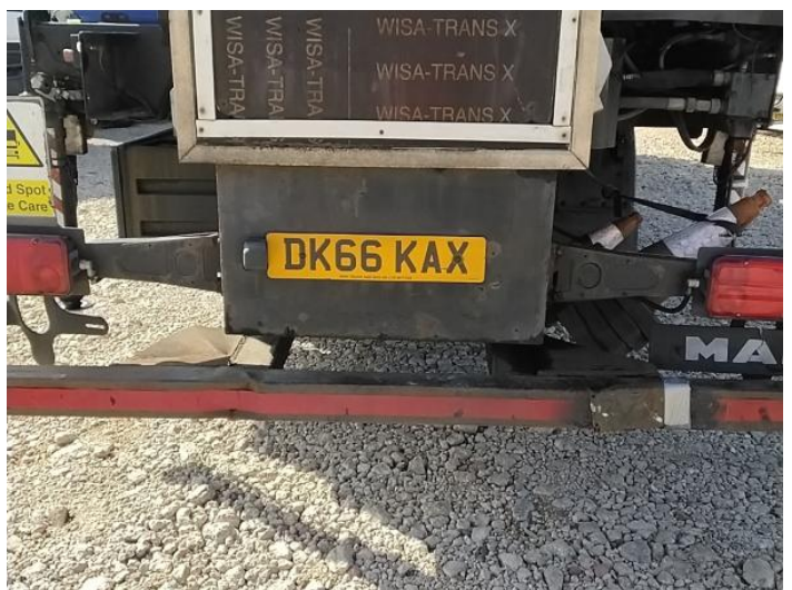
14: Bumper Rear Rusted Over 5mm
