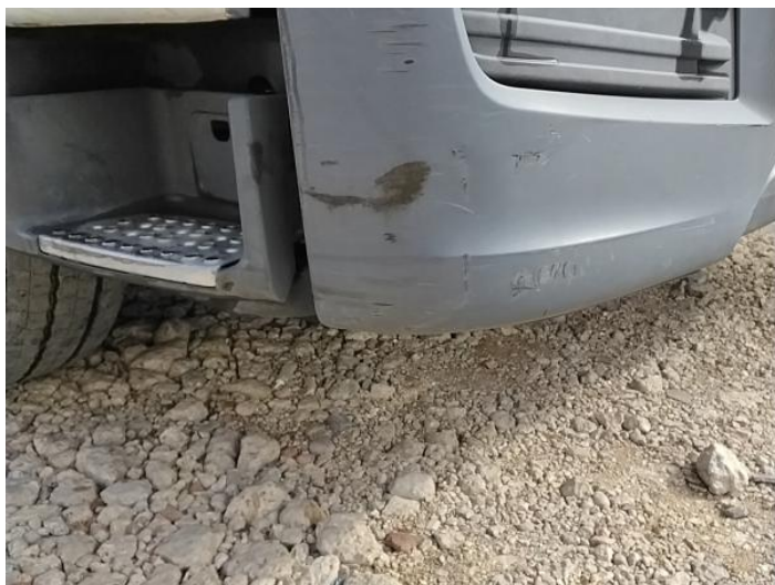
1: Bumper Front Moulding Scuffed (Unpainted) UpTo 100mm
