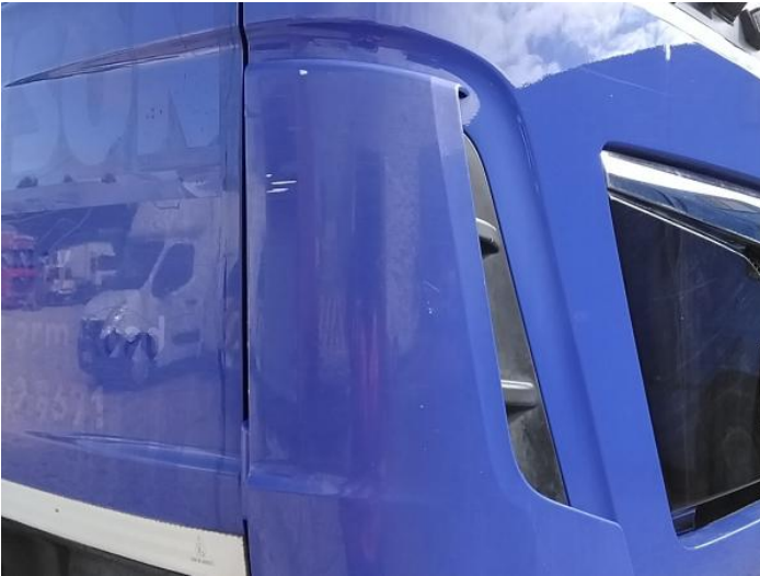
3: Wing osf Scratched UpTo 25mm Thru Paint
