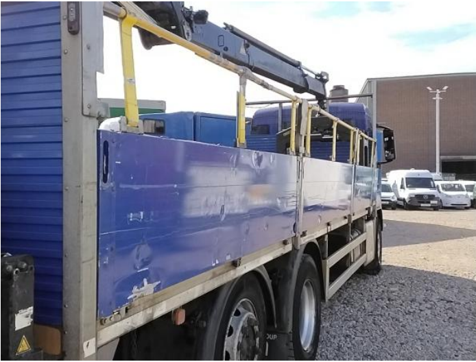
15: Qtr Panel osr Dented Over 30mm
