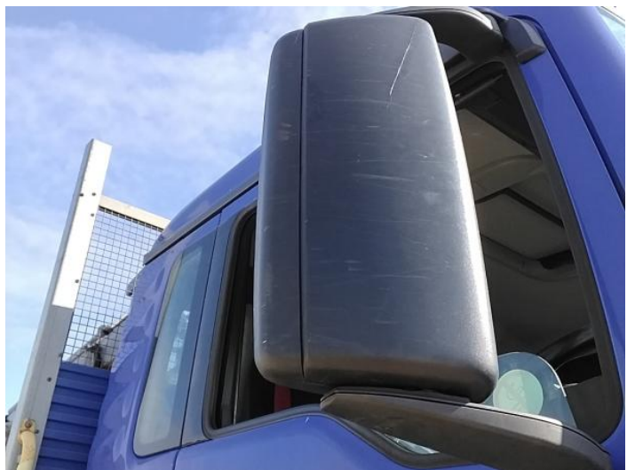
20: Door Mirror Assy osf Scuffed (Unpainted) UpTo 100mm
