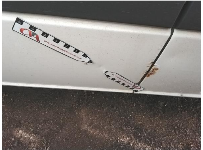
22: Qtr Panel osr Dented Over 30mm
