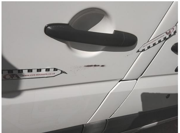
6: Door nsf Scratched Over 25mm Thru Paint
