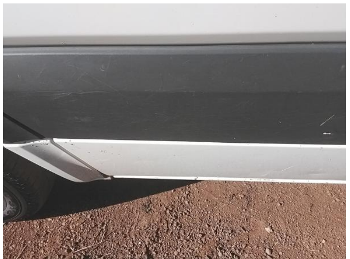
8: Door Moulding nsf Scuffed (Unpainted) Over 100mm
