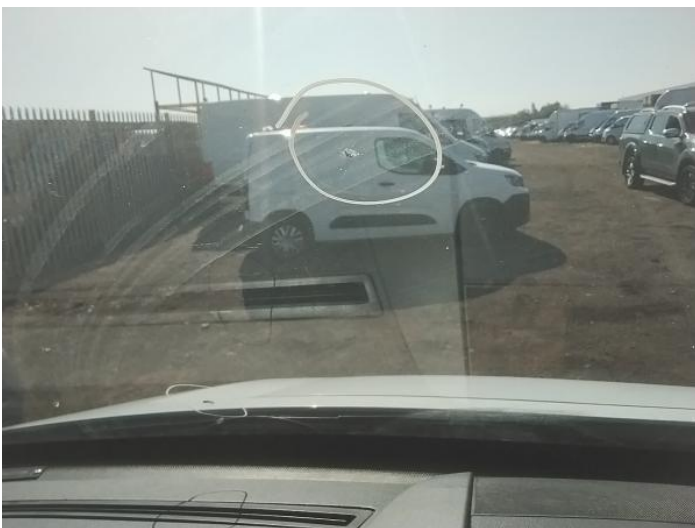
25: Screen Front Chipped Over 10mm
