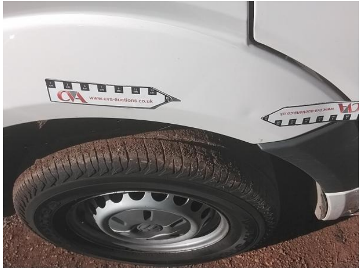
4: Wing nsf Dented Over 30mm
