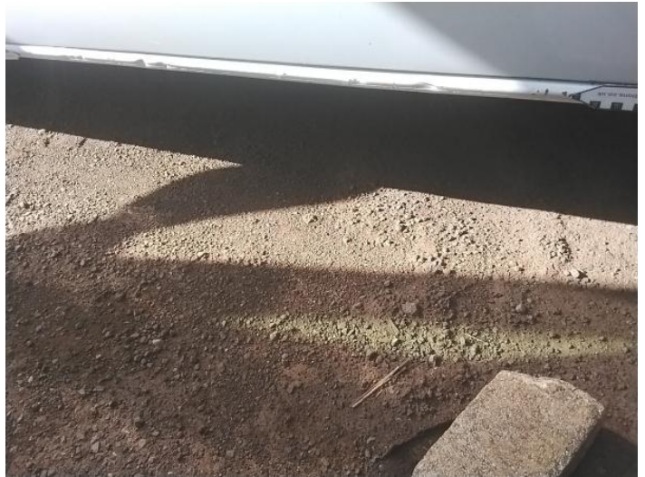
10: Sill ns Dented With Paint Damage
