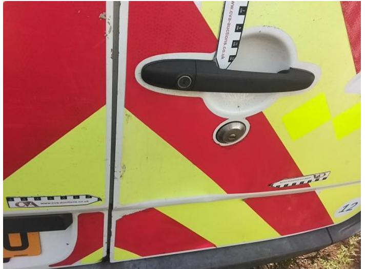
16: Door osr Dented Over 30mm
