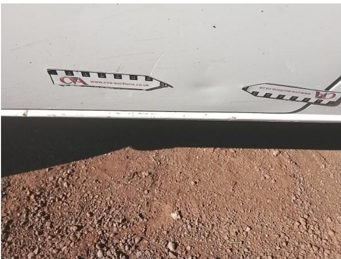
7: Door nsf Dented Over 30mm
