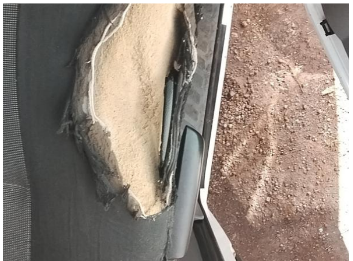
26: Seat Base Cover osf Torn Over 3mm
