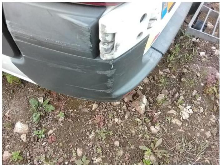
14: Bumper Rear Moulding Scuffed (Unpainted) Over 100mm
