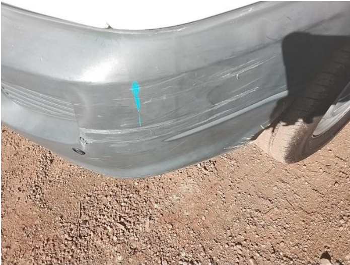
3: Bumper Front Hole UpTo 25mm
