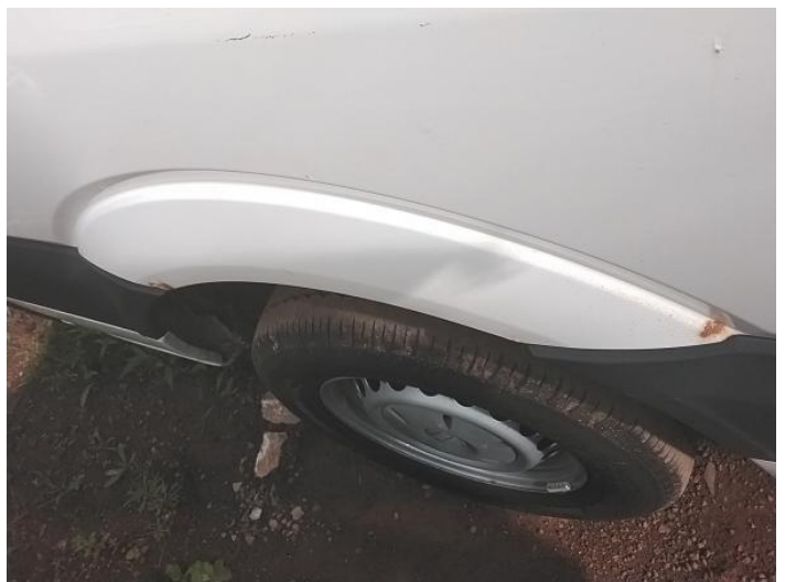
20: Qtr Panel osr Dented Over 30mm
