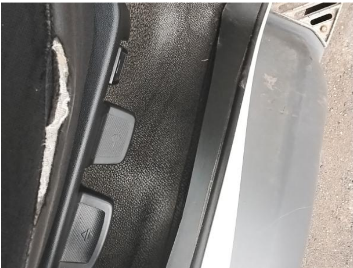
11: Seat Base Cover osf Torn Over 3mm
